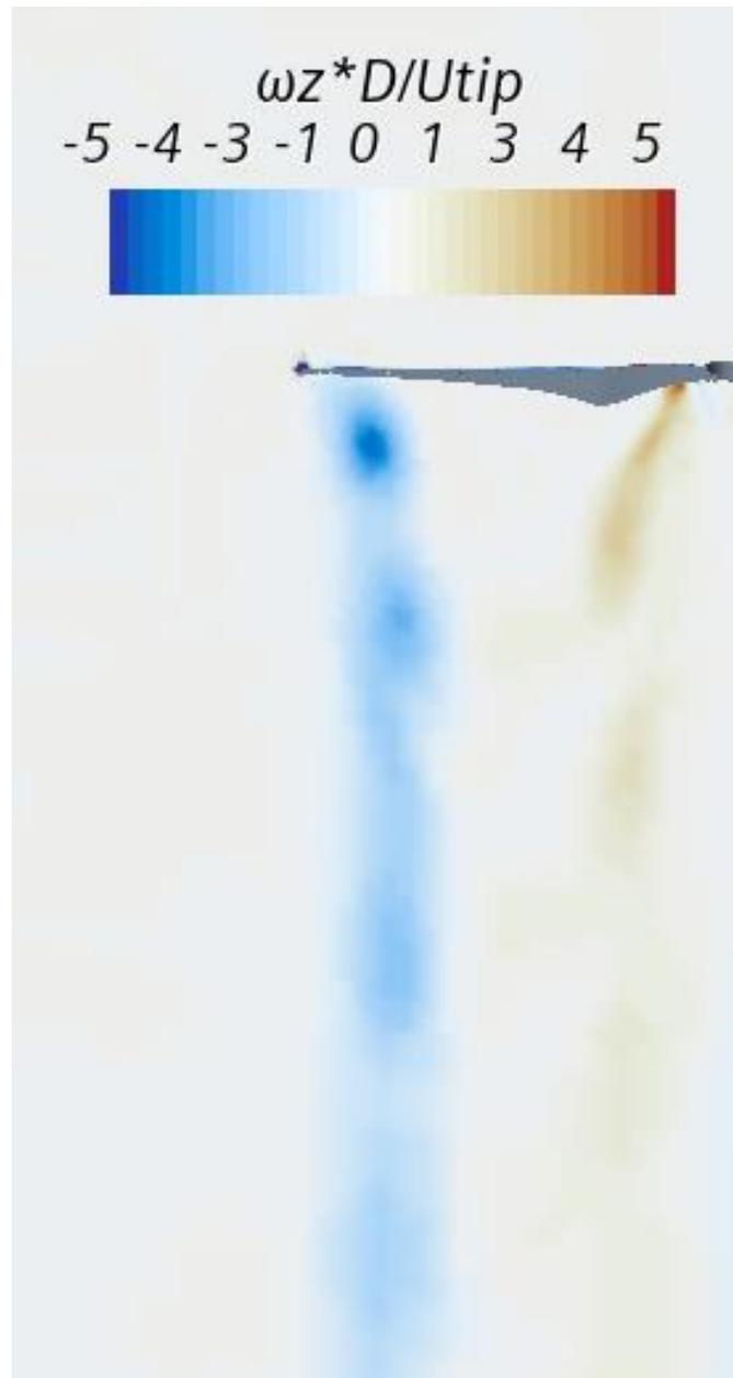
Figure 19: Mean vorticity of 5400 RPM case.
