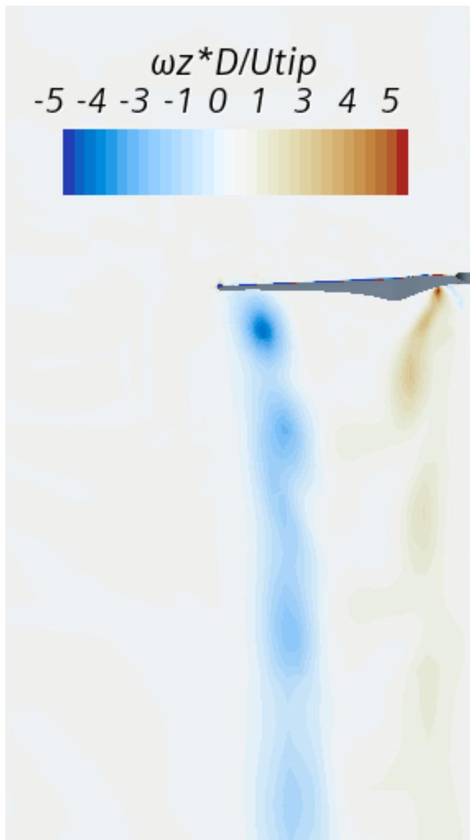
Figure 18: Mean vorticity of 3600 RPM case.
