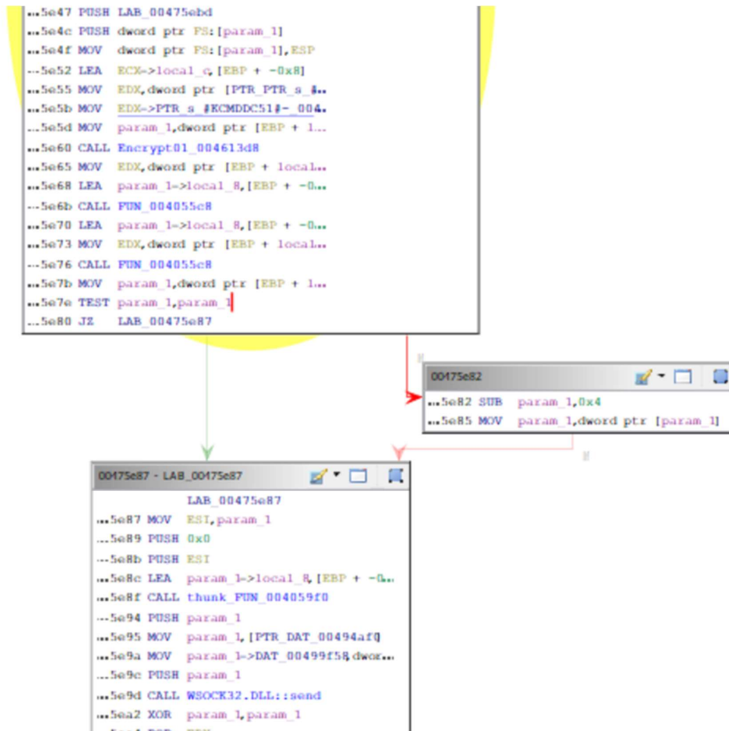
Figure 18 - Key Preceding Send: the key string “#KCMDDC51#...” is used to call Encrypt() before send() is called
