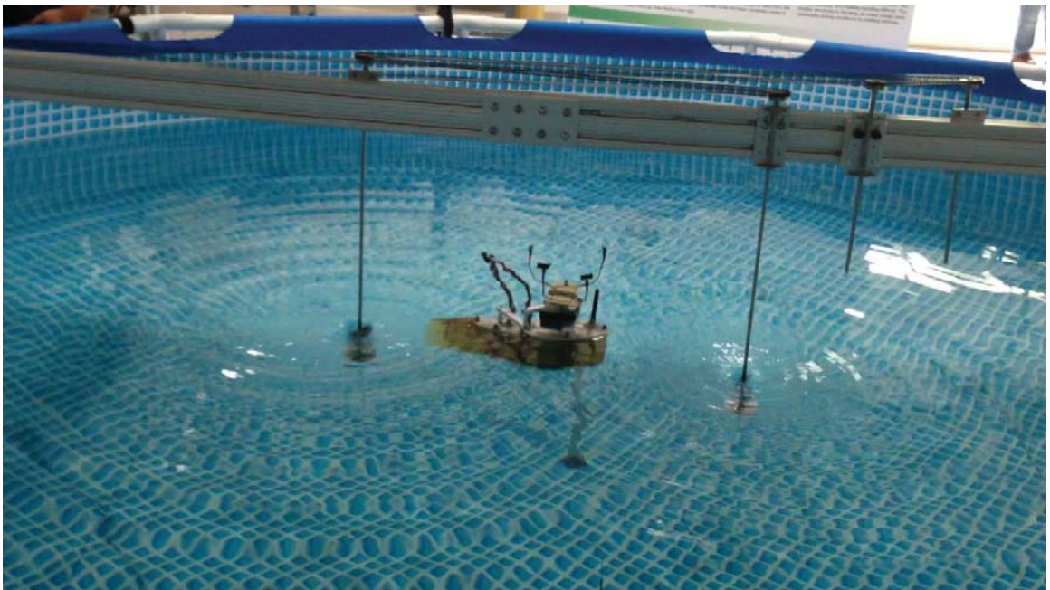
Figure 55: The robot steering through the vortex array.
