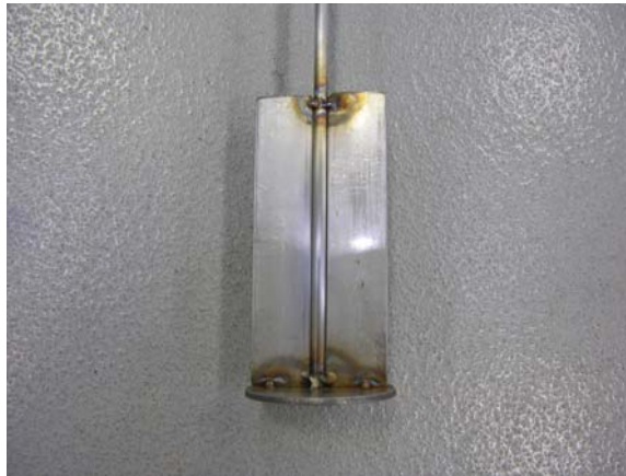
Figure 40: The vortex generator.
