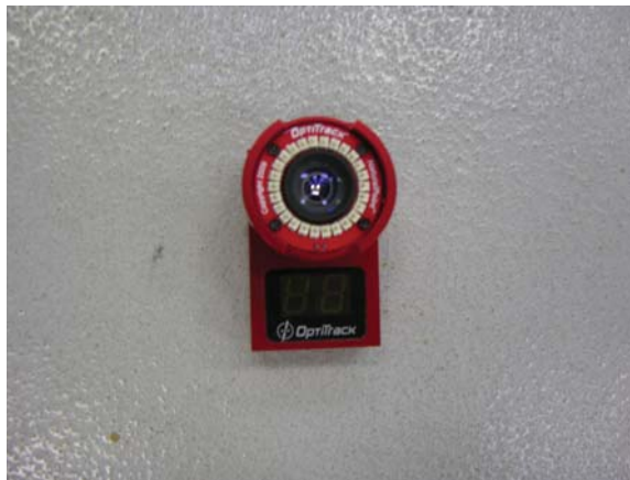
Figure 35: One of six cameras used in tracking the motion of the robot.
