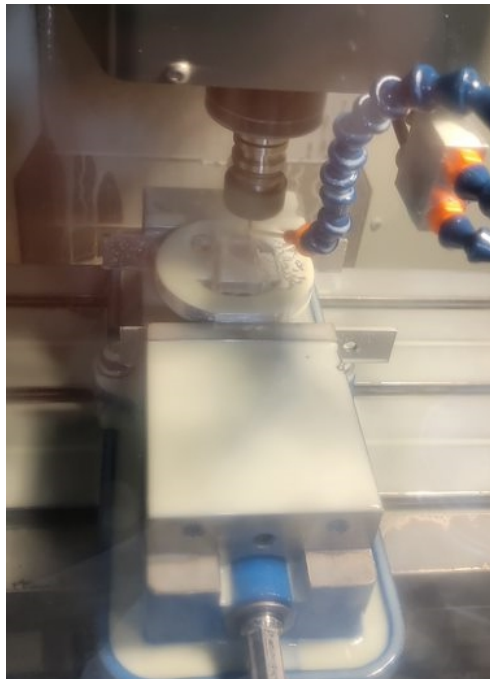
Figure 4.23: Roughing of the optical assembly using the haas tool room mill.
