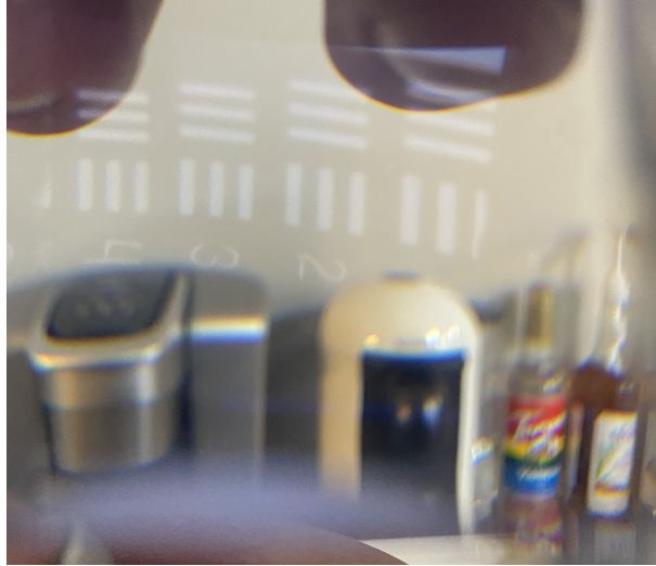
Figure 5.6: Air force test chart imaged by cell phone 2 without a solid background.
