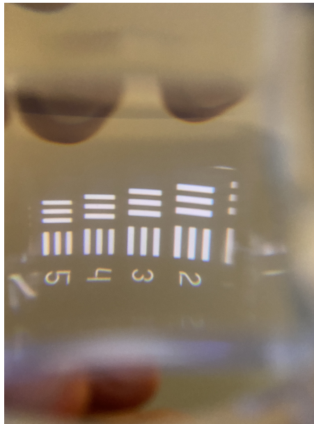
Figure 5.5: Air force test chart imaged by cell phone 2.
