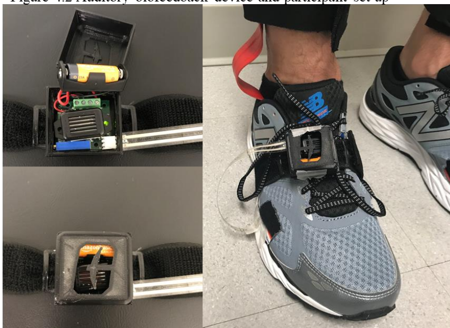
Figure 4.2 Auditory biofeedback device and participant set up
