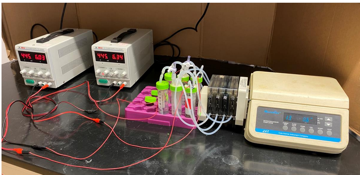
Fig. 3.3 Continuous reactor with recirculation setup used for electrochemical mineralization of GenX
