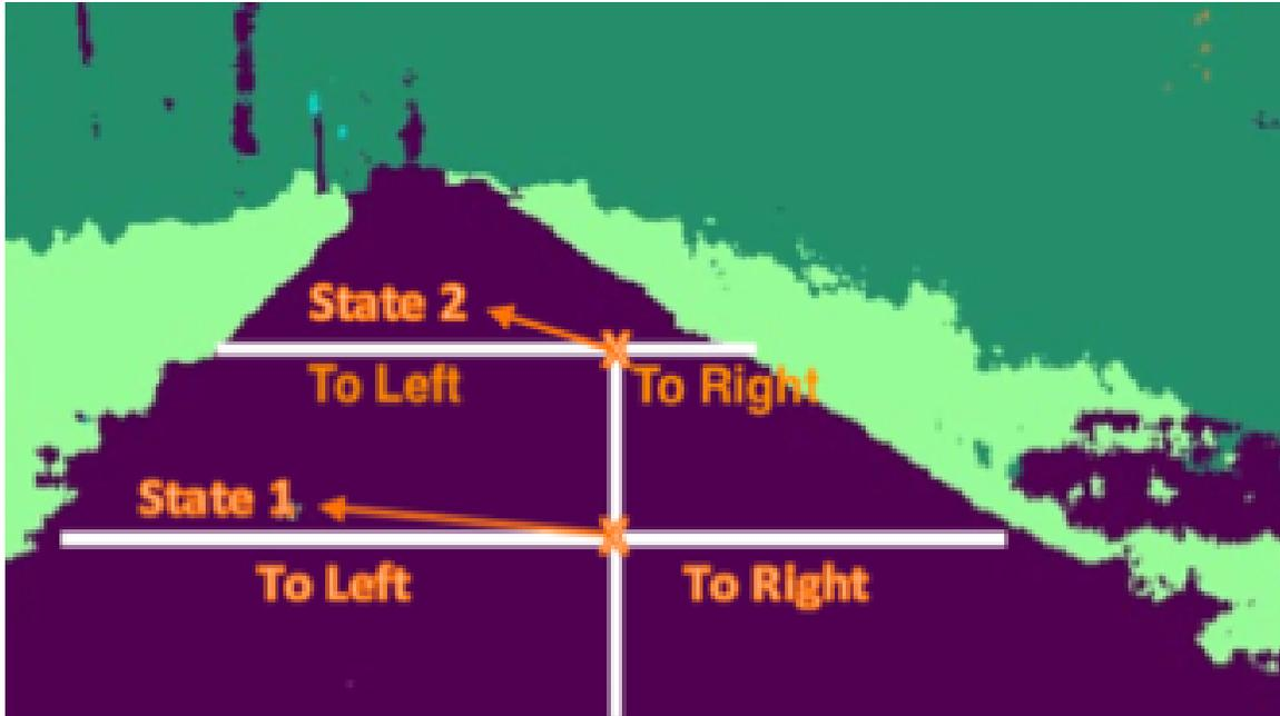
Figure 5.14: ATV current state (State 1) versus ATV trajectory projection state (State 2)
