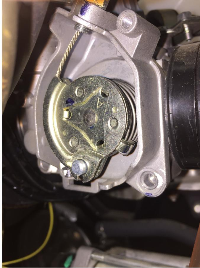
Figure 3.16: Throttle wire and spring at the air valve side
