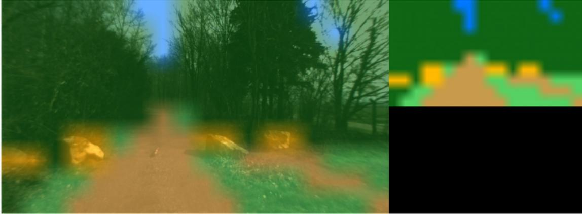
Figure 5.11: Example for the SegNet S.S. [64], on the left it is the overlay of the mask on the original image, while on the right, there is the mask used
