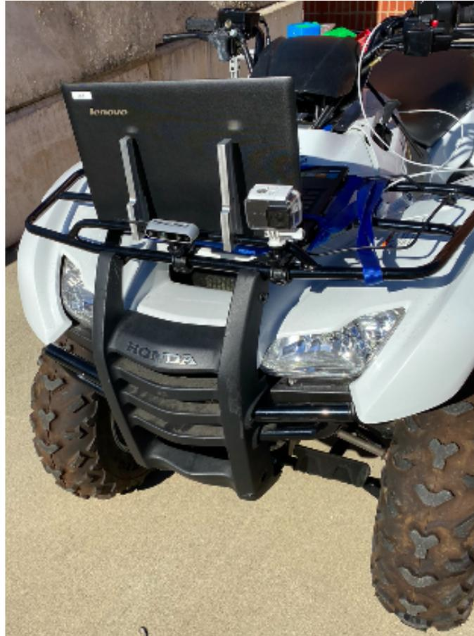
Figure 5.2: The cameras mounted on the ATV
