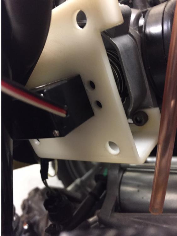
Figure 3.18: Servo motor attached to the air valve controller
