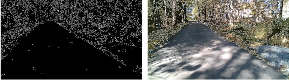
Figure 5.8: Applying edge detection on the color masked frames
