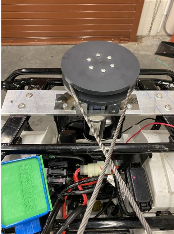
Figure 3.28: Cable driver of the handlebar attached to the pulley in a cross position to increase the range of motion
