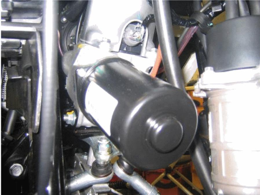
Figure 3.2: DC power steering motor [44].
