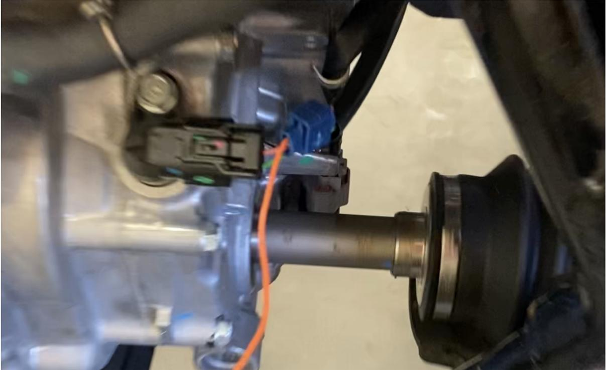
Figure 3.19: Speed sensor attached to the engine
