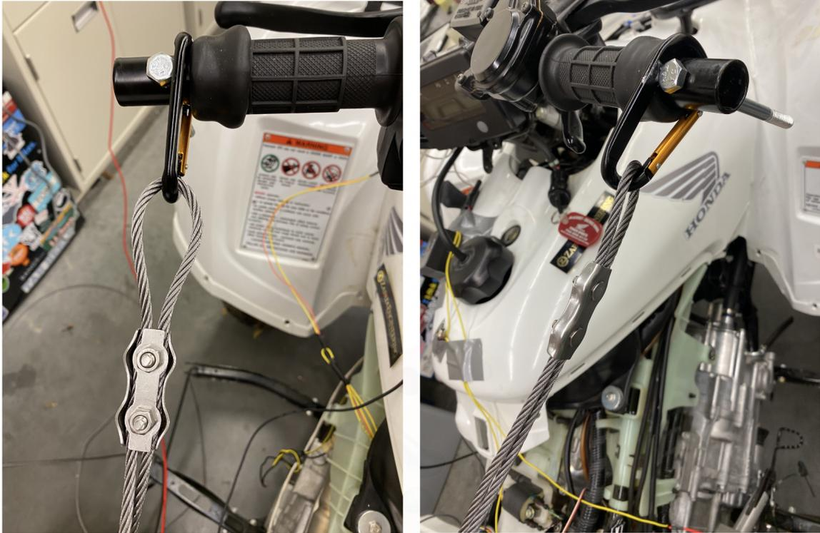
Figure 3.29: Cable driver attached to the handlebar
