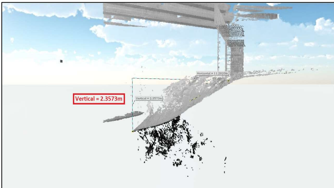
Figure A-5 LiDAR scan image of riverbank deep cut(embankment scour) of Phillips Road bridge
