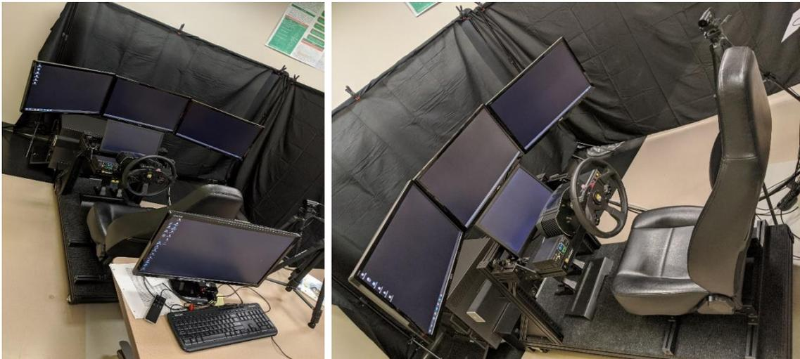
Figure 11 Driver simulator setup
