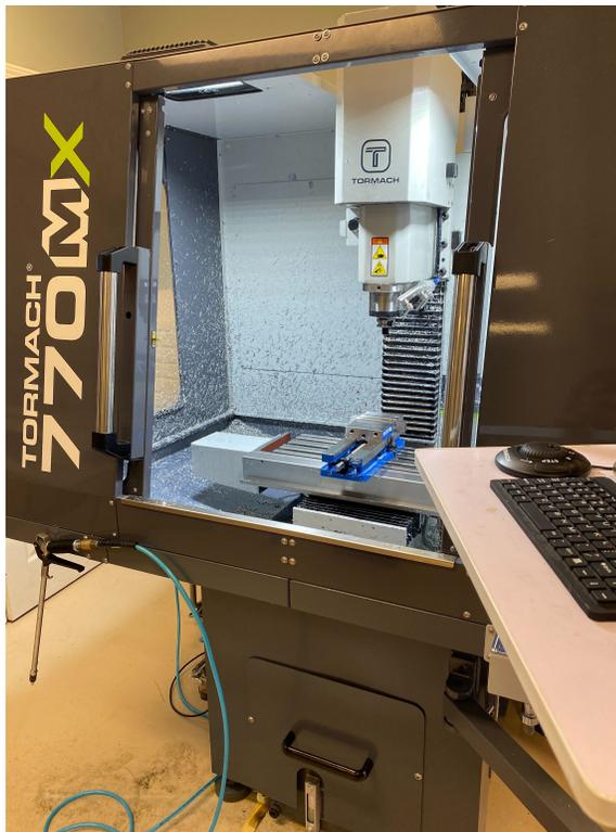
Figure 6.1: Tormach770MX CNC Mill.
