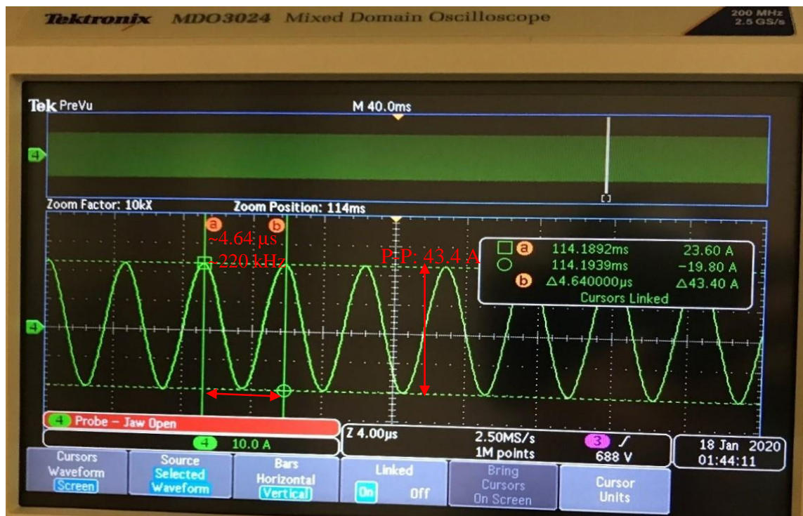
Figure 36. Experimental alternating current measurements of zero voltage switching oscillator circuit using Tektronix current probe (top) and screenshot of the oscilloscope (bottom).
