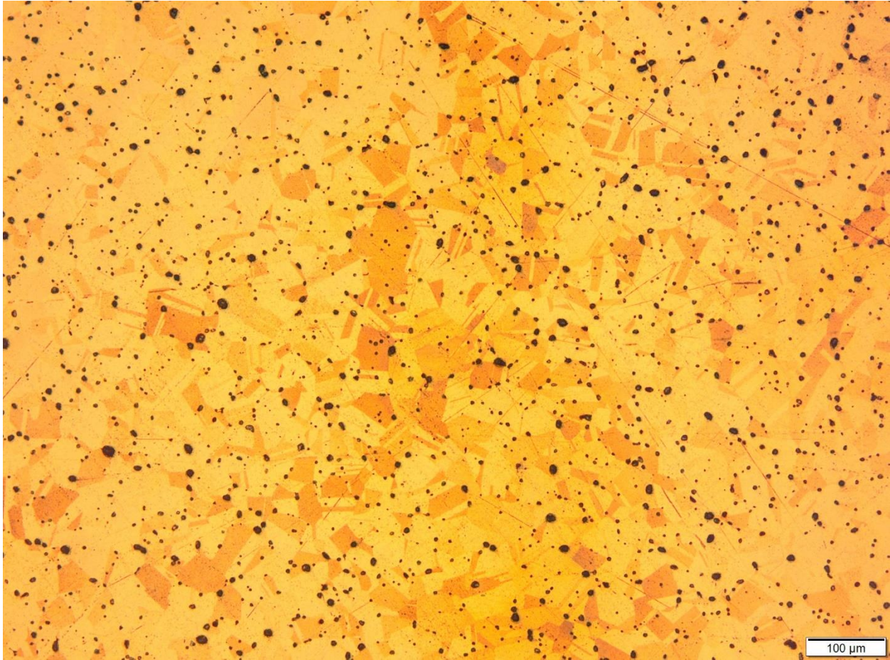
Figure 117. A surface images of an annealed Cu sample with grain size of around 100 \mu\text{m} .
