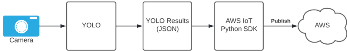
Figure 4.1: Setup for testing Edge processing
