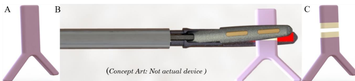
Figure 2.1: (A) A harvested porcine blood vessel. (B) Concept art of a laparoscopic laser-based device to seal and cut a blood vessel with real time feedback. (C) A successfully sealed and cut vessel (not drawn to scale).
