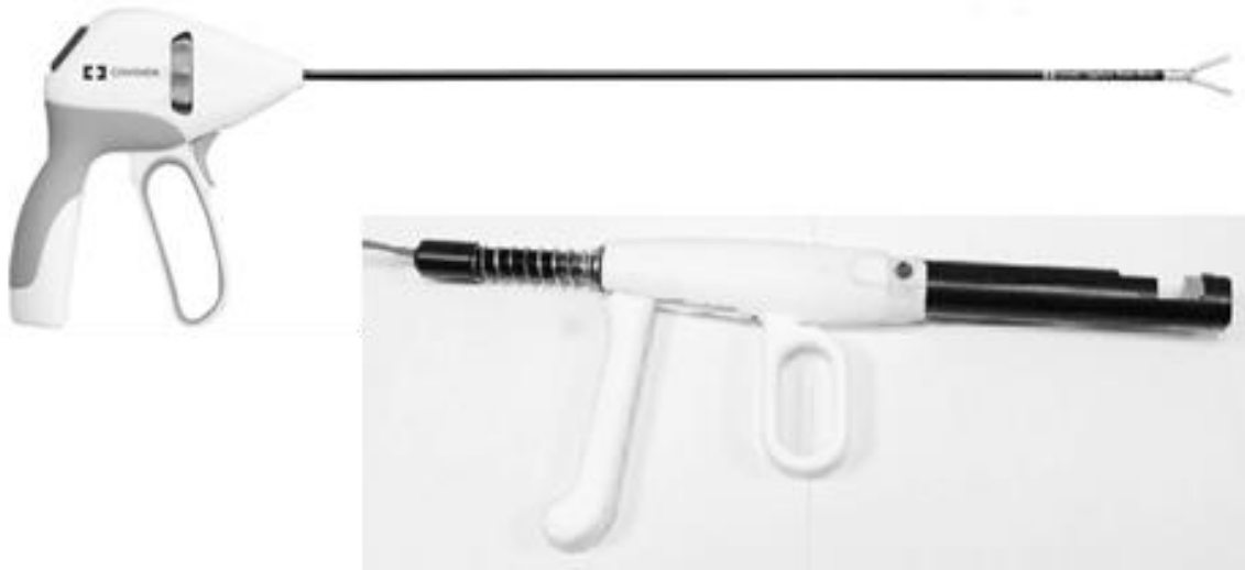
Figure 7.1: (Left) Maryland style laparoscopic RF electro-surgical device, including handle, 5-mm-OD arm/shaft, and jaws for grasping vascular tissue bundles. (Right) Open surgical infrared laser vessel sealing device, featuring a plunger style tissue clamping mechanism in a cylindrical head with 1/2 inch (12.7-mm-OD) components, too large for laparoscopic surgery [82].
