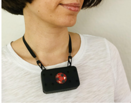
Figure 2.2: Application of the developed spectrometer presented in this study for measuring personal light exposures.
