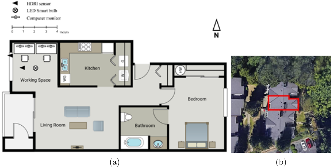
Figure 3.2: Example of home-office layout. a) plan shows where the subjects were seated, positions of computer monitors, LED smart bulb, locations, and view orientations of HDRI sensors, b) surrounding urban context.
