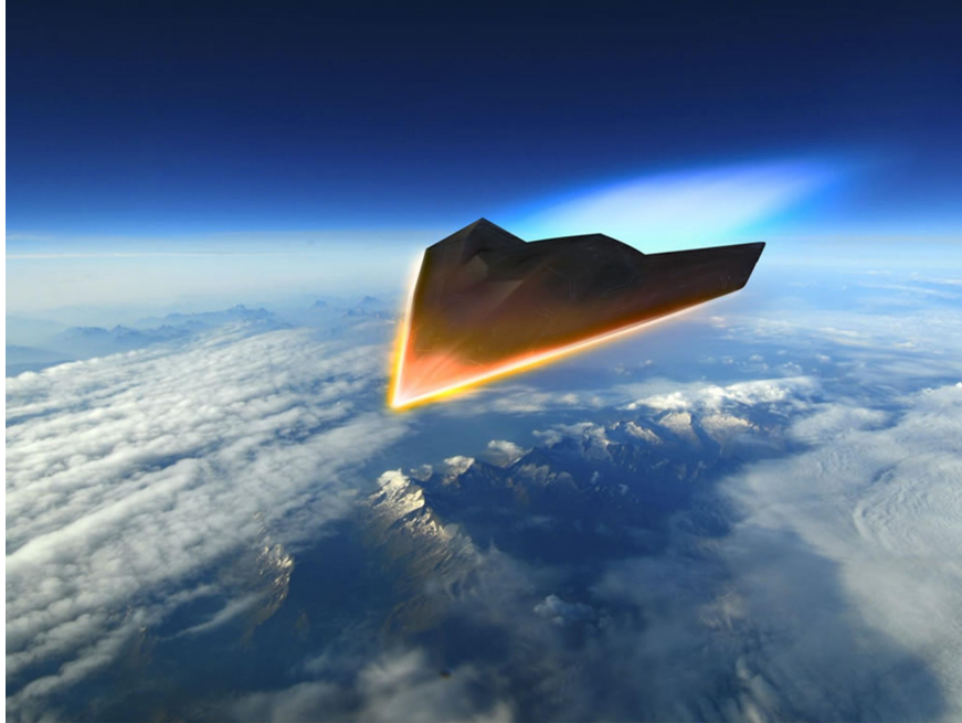
Figure 1.1: Hypersonic Glide Vehicle, Leading Edges Experiencing High Friction and Heat Loading
