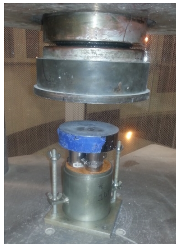
(c) pushing tubes into the soil sample
