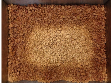
(a) sample preparation, breaking clogs, adding water to reach designated moisture
