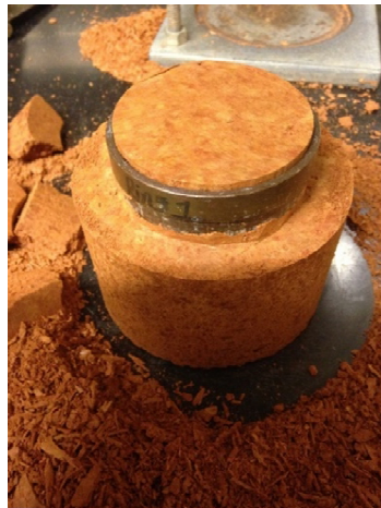
(c) trimming off soil outside the oedometer ring
