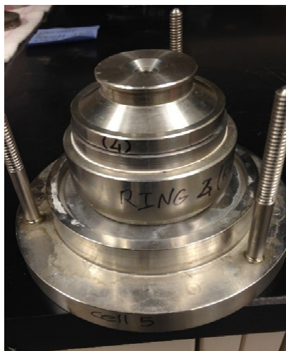
(e) placing filter papers on top and bottom, steel disc and loading pad on top of the specimen
