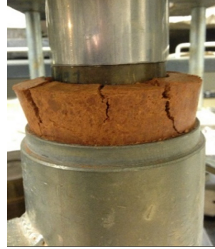
(b) compaction test and pushing the solid ring
