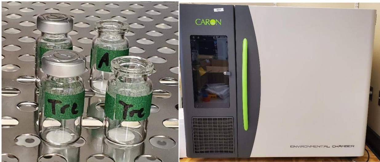
Figure 4. Storage vials and environmental chamber. One of each of the paired samples was opened and the other left sealed for treatment (left). Adverse conditions of 76% RH were induced by the environmental chamber (right).
