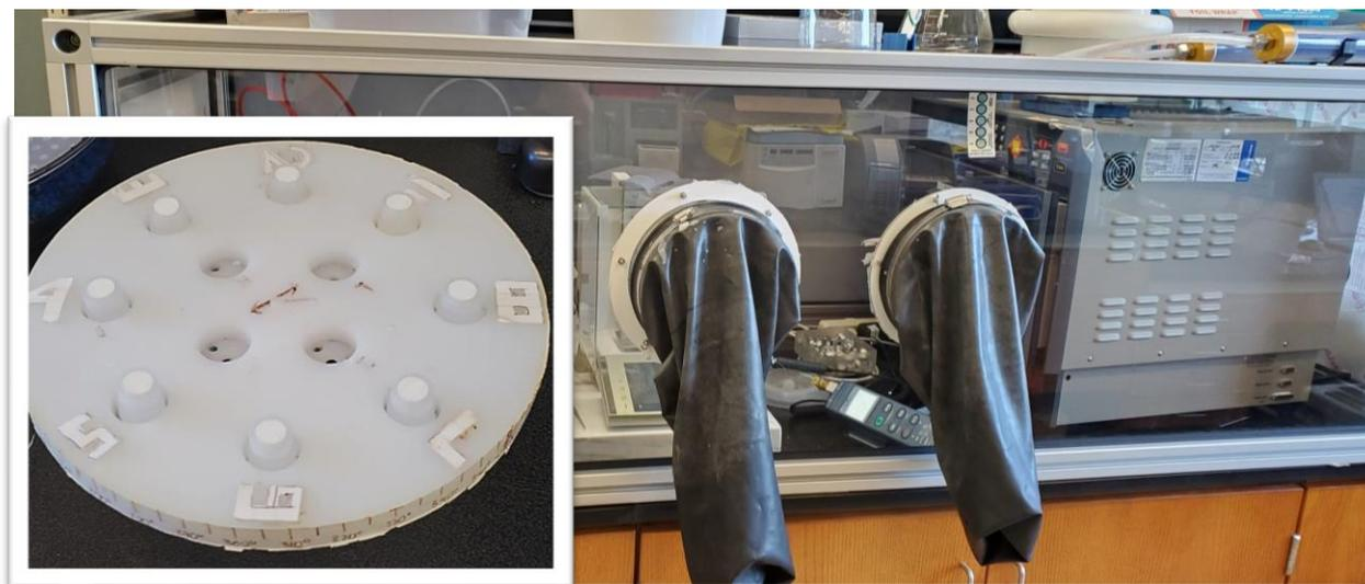
Figure 1. Controlled humidity chamber and microwave setup. The microwave turntable set up to hold 8 samples atop syringe filter holders (inset). Controlled environment chamber with attached access gloves, containing microwave, balance, and Karl Fischer Titrator (background).
