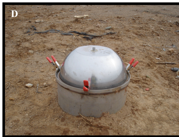
Figure 31. Flux chamber configuration. A) Diagram of flux chamber. B) Photo of flux chamber components. C) Photo of biotarp prototype in flux chamber. D) Photo of assembled flux chamber.
