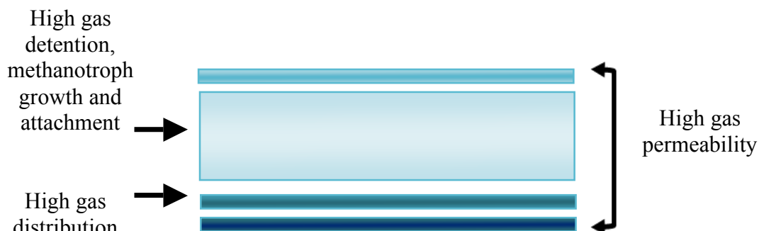
Figure 37. Ideal biotarp prototype based on results from continuous flow chamber trials.
