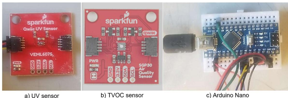
Figure 24: Air quality, UV light Sensor, and Arduino Nano
