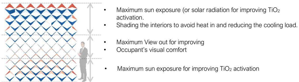
Figure 12: Design Intent for facade panel
