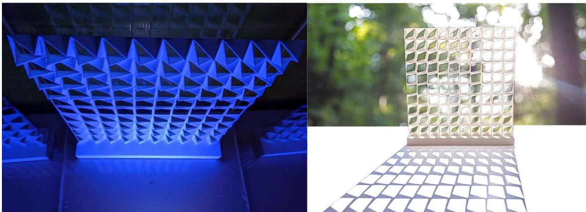
Figure 10: 3d printed facade panel (b)
