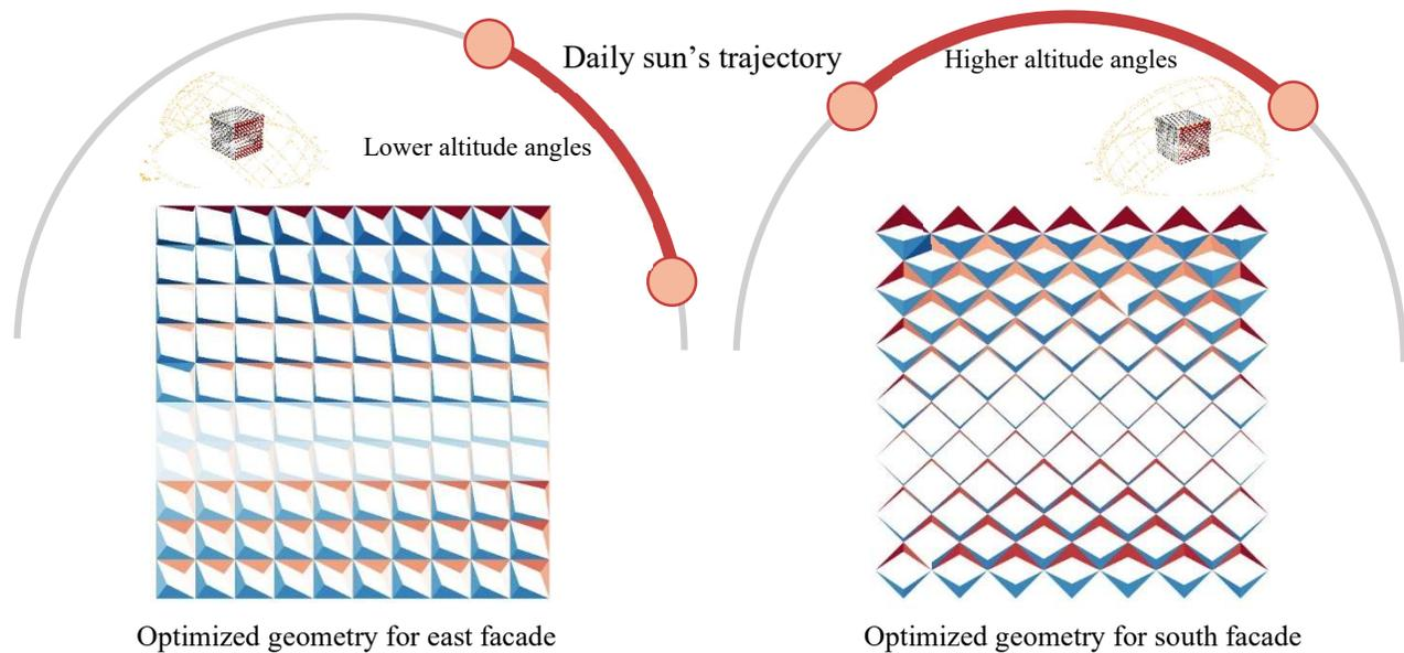
Figure 16: Design Intent for facade geometry on east and south façade
