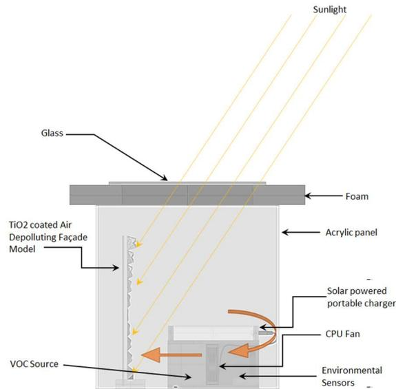
Figure 23: Testing Chamber - Side View
