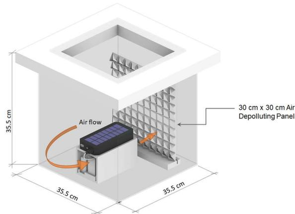
Figure 22: Testing Chamber – Isometric View
