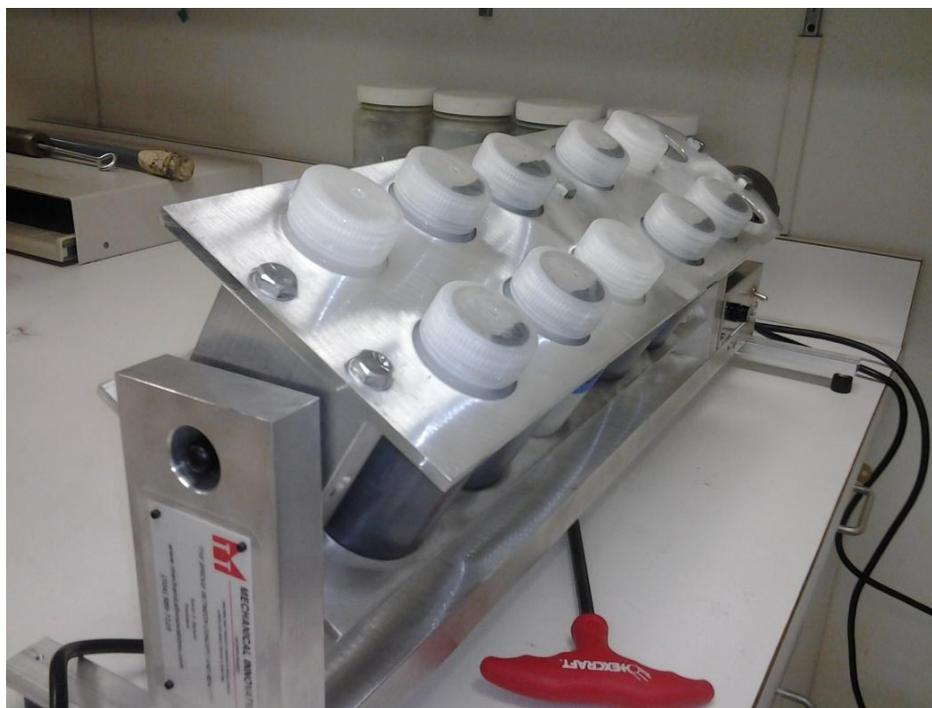
FIGURE 6-1: pH dependence test experimental setup
