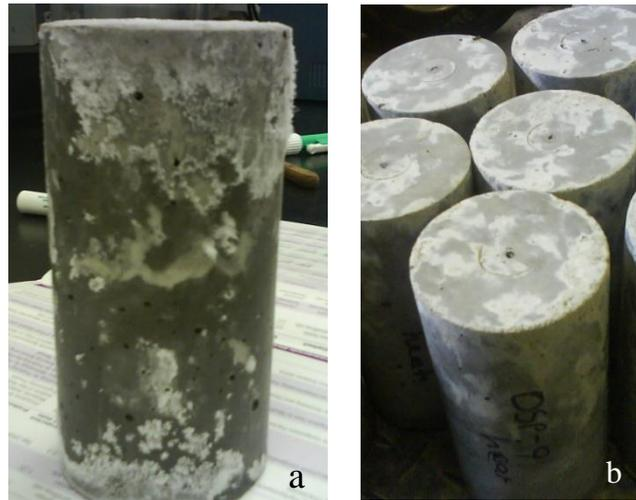
FIGURE 4-6: Cured geopolymer concrete a) cured without heat, b) heat cured
