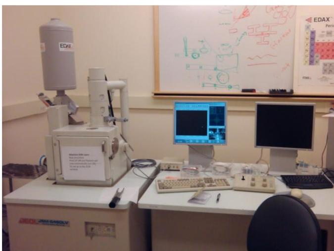
FIGURE 7-7: JOEL SEM equipped with energy dispersive spectrometry (EDX)
