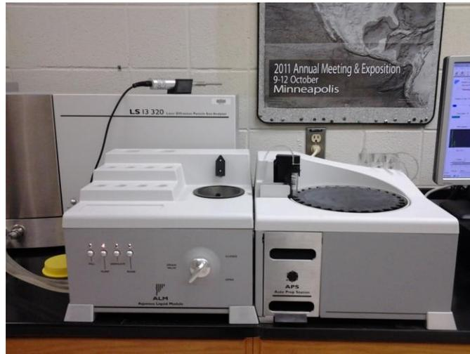
FIGURE 5-2: Laser diffraction particle size analyzer
