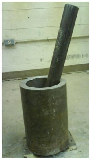
FIGURE 4-2: Steel pestle and mortar used in crushing the geopolymer concrete
