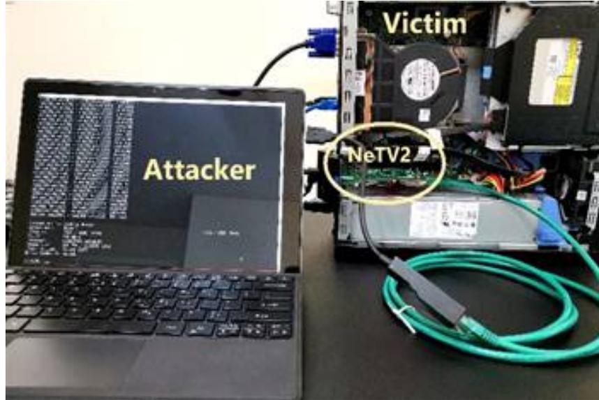
Figure 3.1: Setup for the PCIIeech attack.
