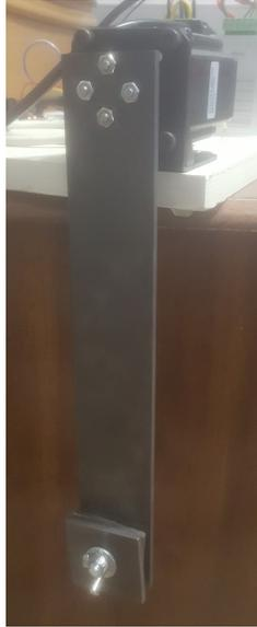
Figure 4.12: Simulated prosthetic thigh load.
