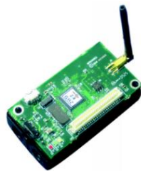
Figure 6.2: Shows a Micaz Mote with radio platform MPR2400 based on the Atmel ATmega128L [65].
