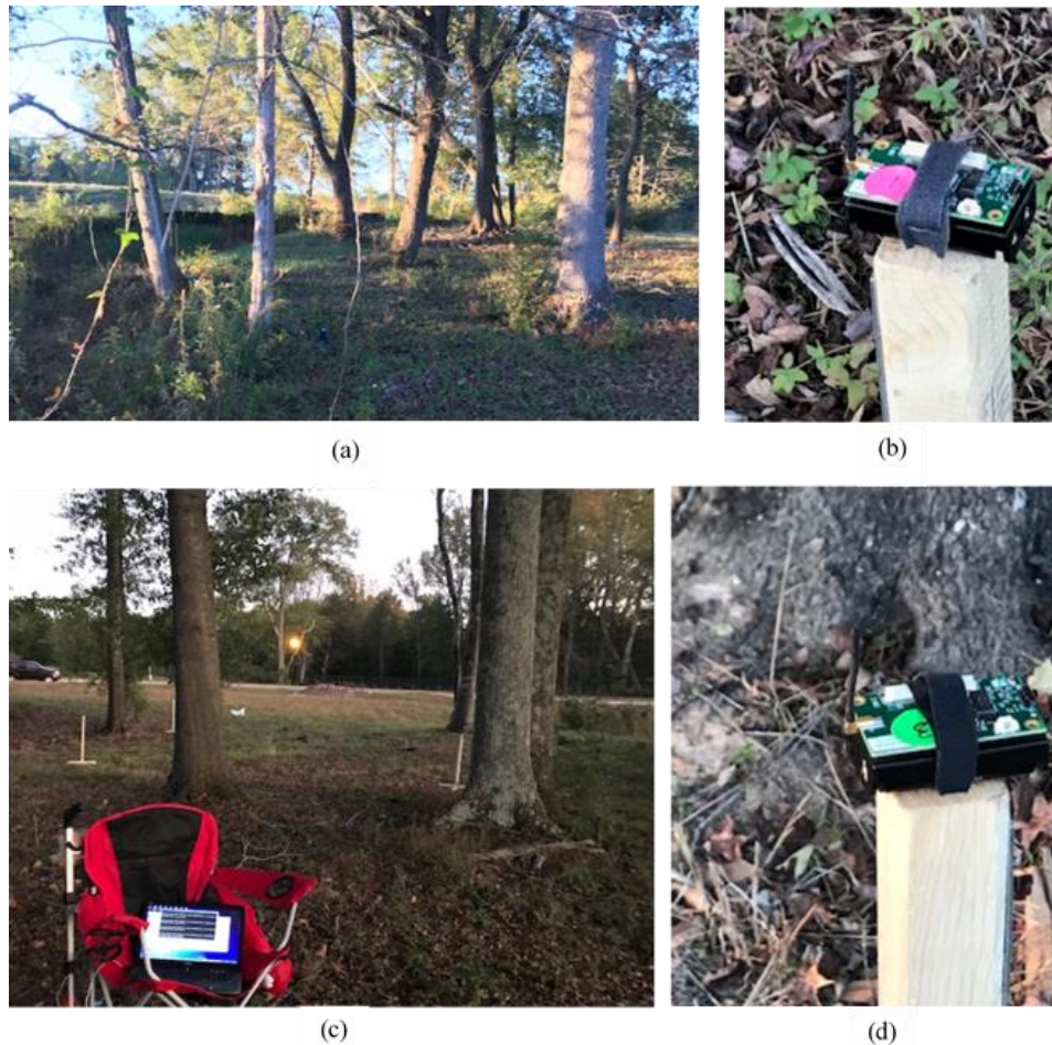
Figure 6.5: Wooded location in Simpsonville, SC. (a) Cross section of the wooded area showing trees and shrubs, (c) deployment area showing the stands on which the sensor nodes: BNs and UNs are mounted on, (b) & (d) shows UN1 and UN3 mounted on top of stands to elevate the height of the deployed sensor nodes.
