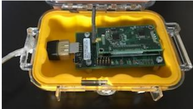
Figure 6.6: Shows the MIB510 Mote Interface Board used in our experiments and a base station connected to it.
