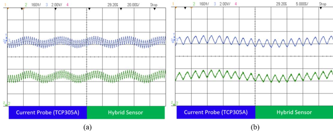
Figure 3.15: Performance of the proposed wideband AMR-Rogowski current sensor in measuring high frequency inverter output current compared to a current probe: (a) regular and (b) zoomed
