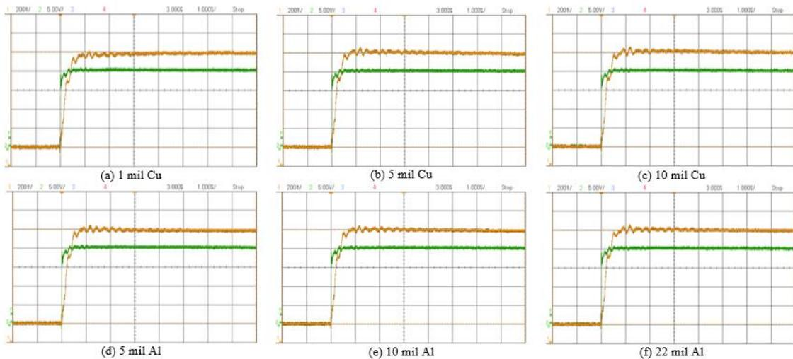
Figure 2.11: Improvement in the response of the AMR sensor with respect to 20A step current with 6 different MCONs. Scales - X-axis: 1 $\mu$ s/div, Y-axis: 5v/div (green), 200mv/div (yellow)
