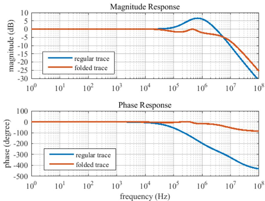
Figure 1.8: Frequency Analysis (normalized) of AMR sensor with Regular (Bare) Trace and Folded Trace based on the experimental results shown in Figure 1.7.
