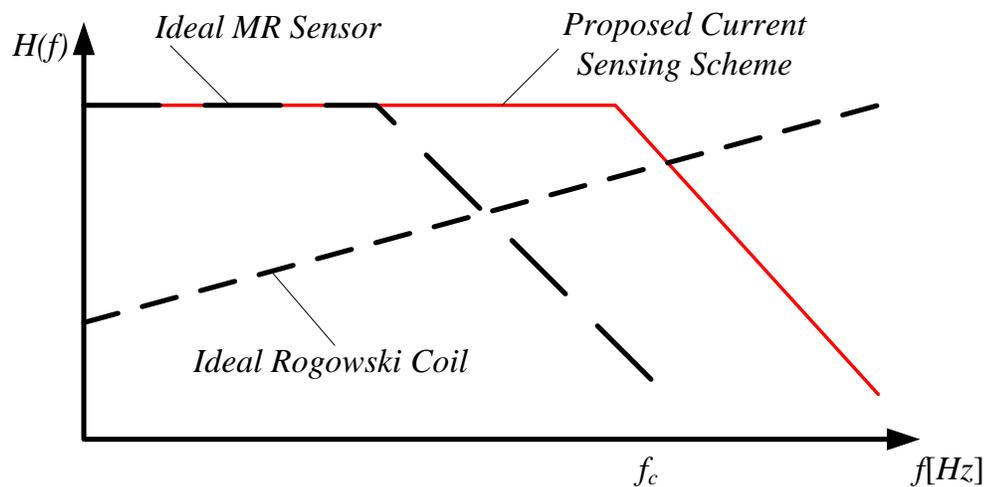
Figure 3.2: The proposed AMR-Rogowski hybrid current measurement scheme.
