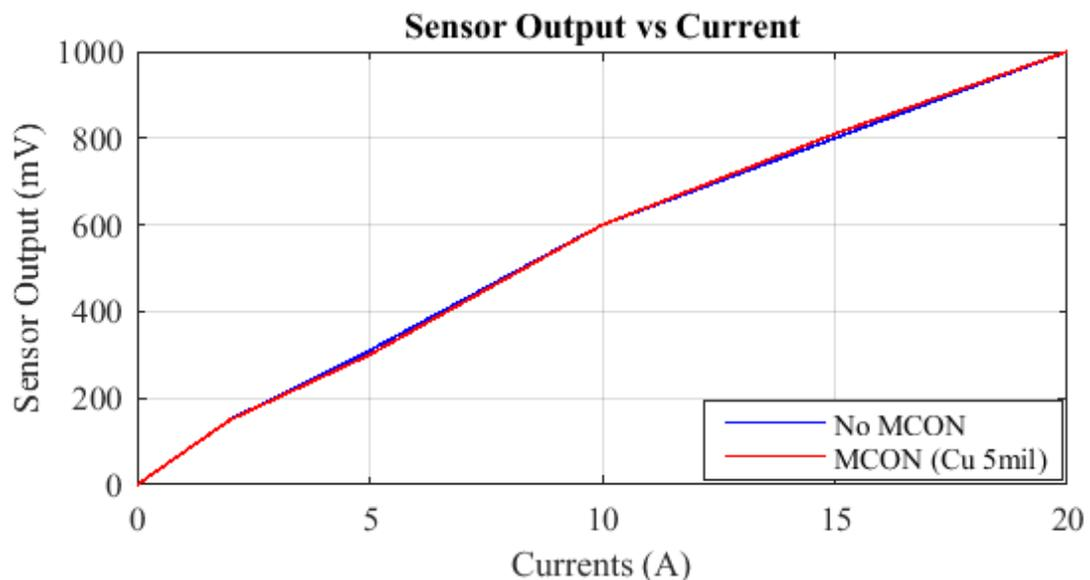
Figure 2.13: Change (offset 2.5V) in steady state sensor output with step currents of different magnitude for no MCON and 5 mil copper MCON
