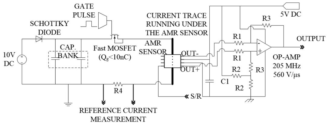
Figure 2.4: Circuit diagram of the hardware setup for evaluation of the performance of the AMR sensor equipped with different MCONs.
