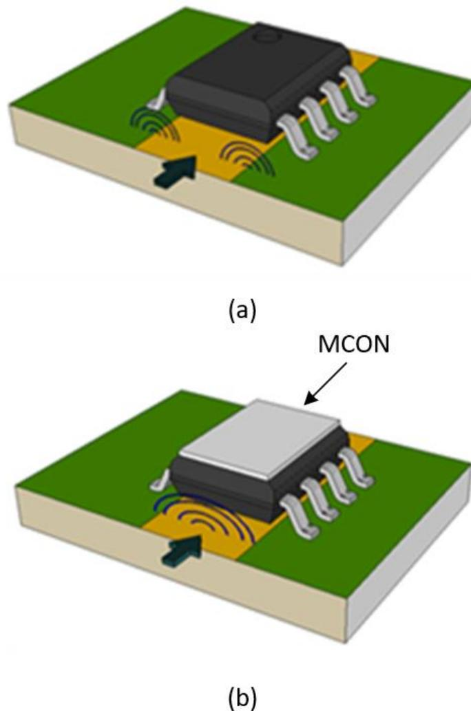
Figure 3.4: Planar Magnetic Concentrator (MCON) concept: (a) Magnetic field distribution at high frequencies due to skin effect and (b) Magnetic field distribution with MCON
