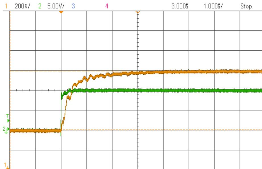
Figure 2.7: Response of the AMR sensor with respect to 10A step current with no MCON. Scales - X-axis: 1µs/div, Y-axis: 5v/div (green), 200mv/div (yellow)
