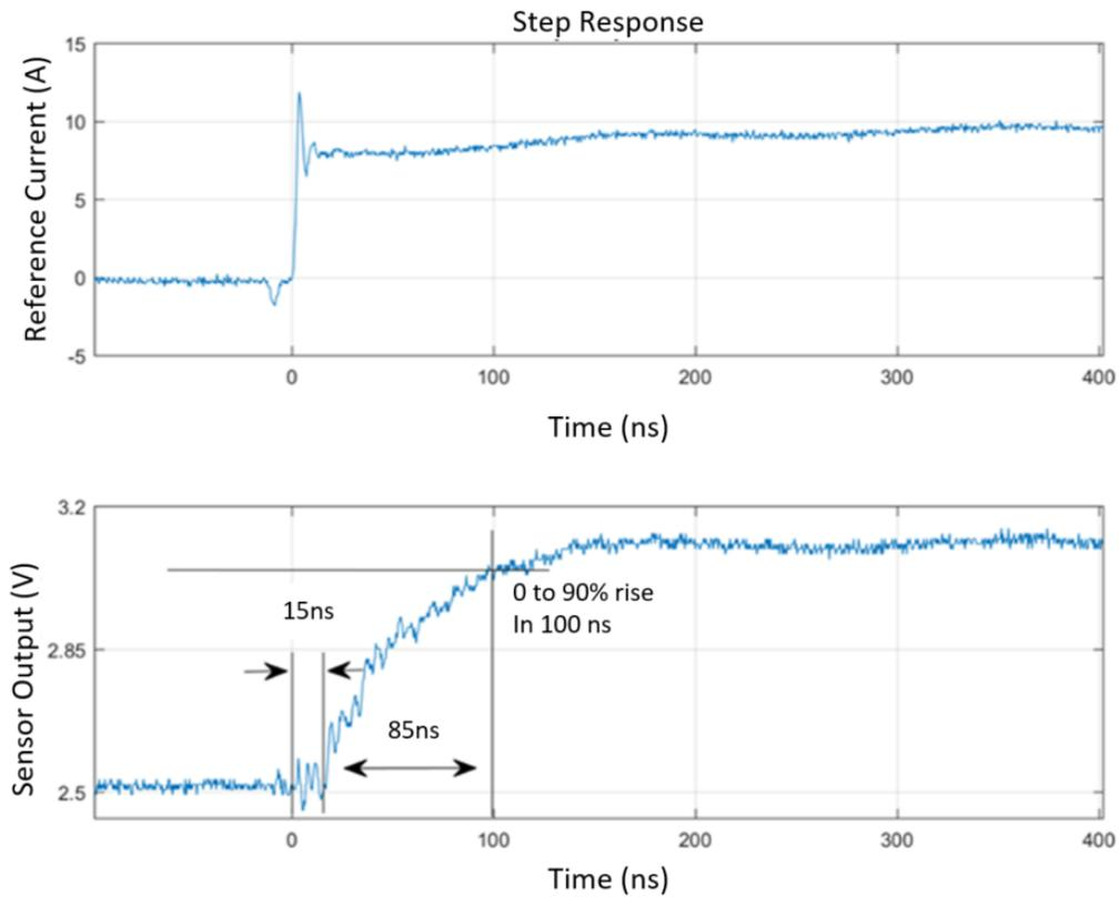
Figure 3.12: Hybrid sensor response for 10A step current (zoomed).
