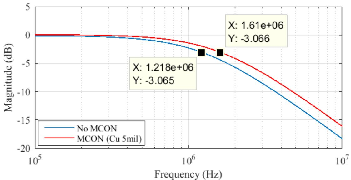
Figure 2.15: Frequency response showing the bandwidth improvement for the step current response presented in Figure 2.12 for no MCON and 5 mil copper MCON
