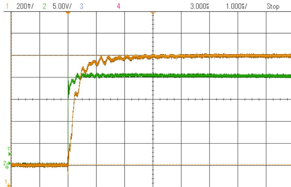
Figure 2.10: Response of the AMR sensor with respect to 20A step current with no MCON. Scales - X-axis: 1 $\mu$ s/div, Y-axis: 5v/div (green), 200mv/div (yellow)
