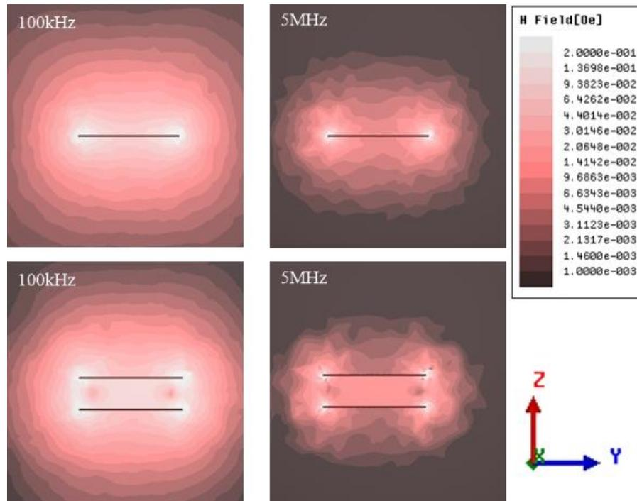
Figure 1.3: Simulation results: magnetic field distribution of bare trace (top) and folded trace (bottom) at two different frequencies.
