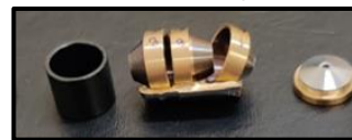
Lens assembly taken from a 60X obj. lens
