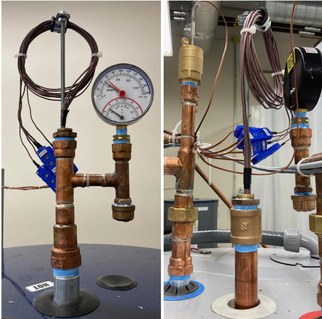
Figure 29: Specially Constructed Vertical Sensor Wells and Thermocouple Probes, Buffer Storage (left), DHW Tank (right)
