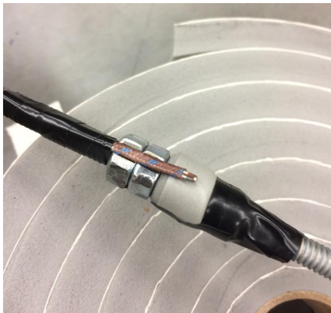
Figure 70: Thermocouple Probe Construction - Transition Joint Fitment
