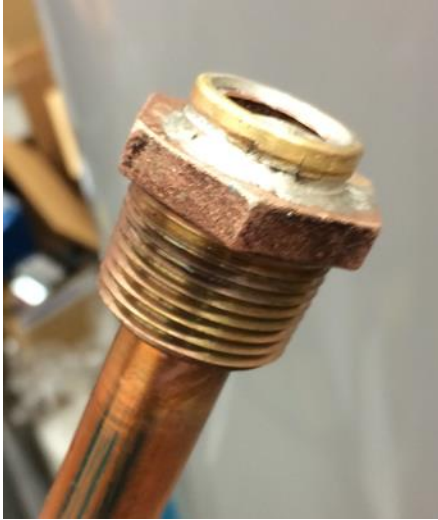
Figure 68: Sensor Well Construction - Soldered Marvel Adapter and Brass Reducing Bushing
