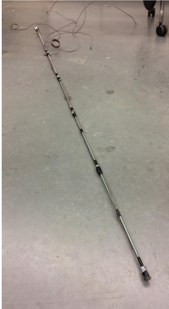
Figure 71: Assembled In-Tank Thermocouple Probe
