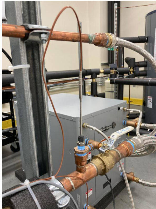
Figure 28: Rugged Transition Joint Thermocouple Probe
