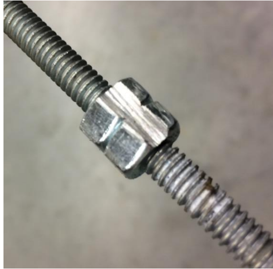
Figure 69: Thermocouple Probe Construction – Counter Tightened Guide Nuts
