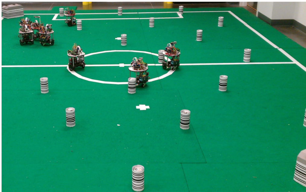
Figure 2.3: Multiple robots path optimizing by moving physical beacons [2].
