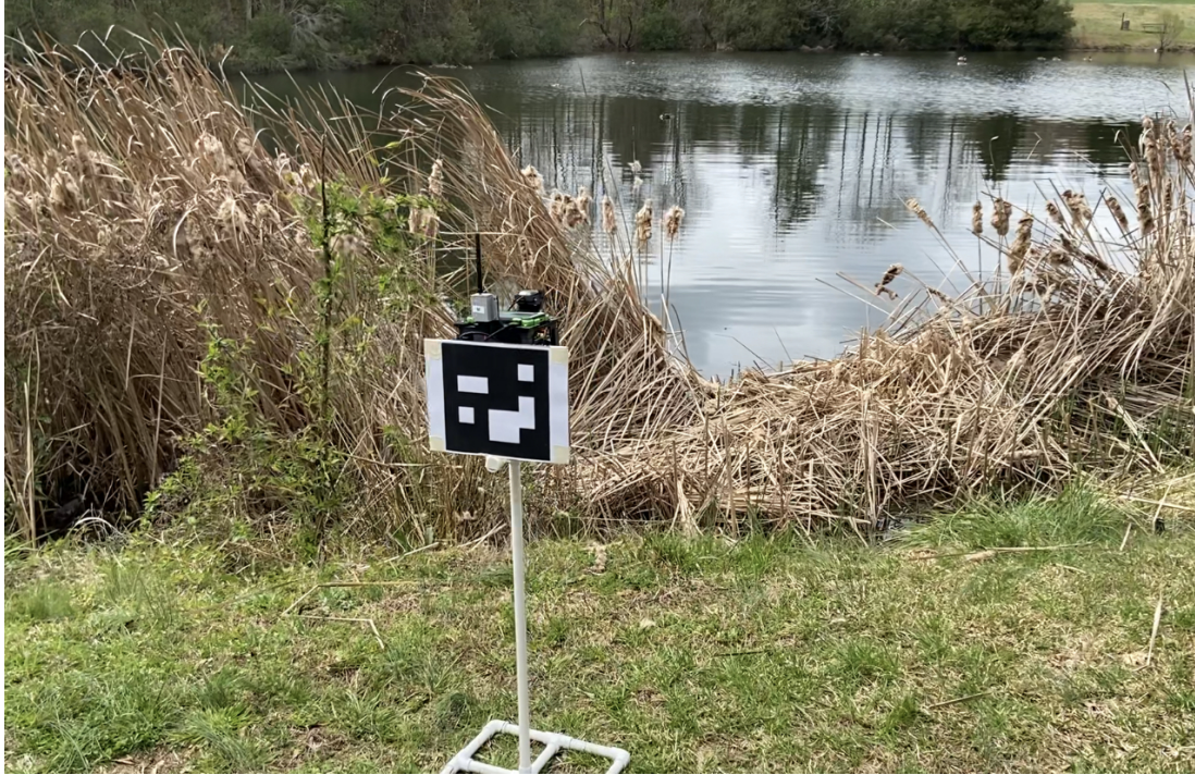
Figure 4.28: Mobile BreadCrumb mounted on PVC pipe to be used for outdoor data gathering.
