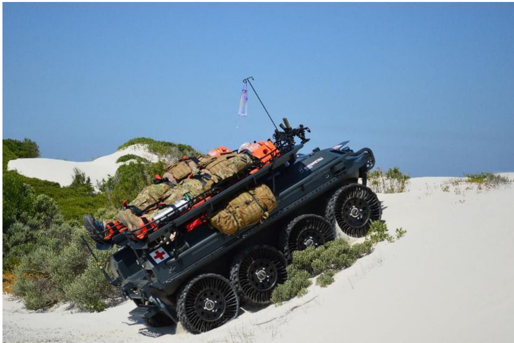
Figure 2.2: Robot rescue vehicle developed by Rheinmetall [1] which can autonomously evacuate casualties over long distances.
