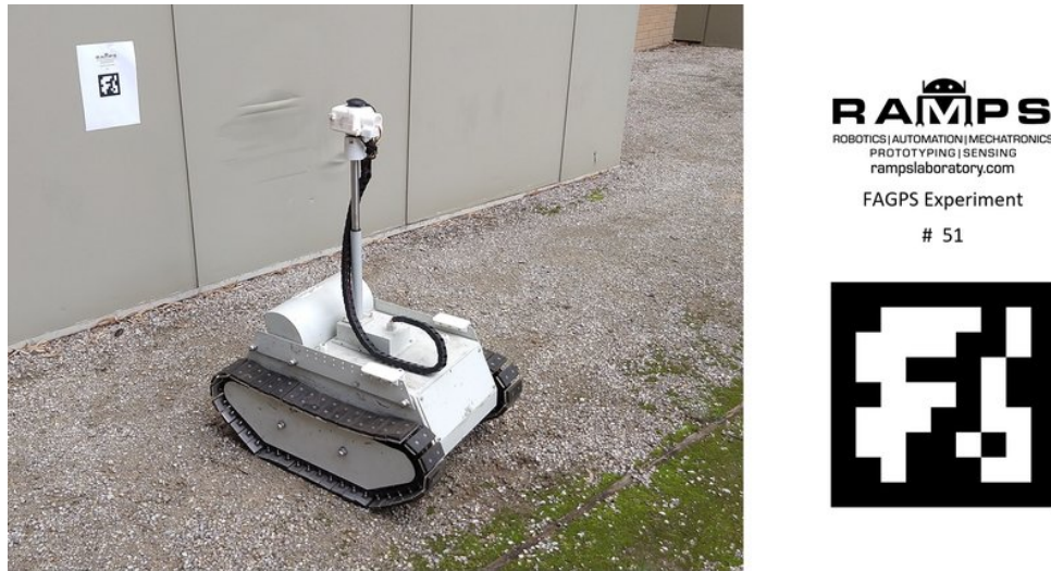
Figure 2.4: Robot observing Fiducials to augment GPS [3].
