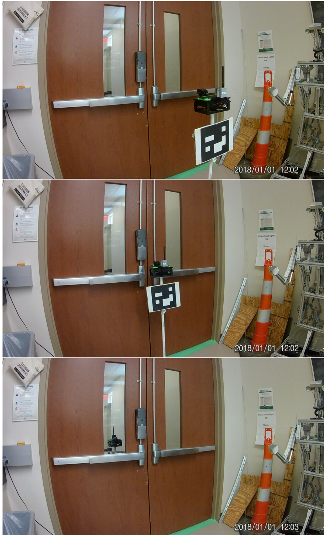
Figure 4.8: Visualization of arUco tag moving through door as measurements are taken. (Note the annotated dates are not meaningful)
