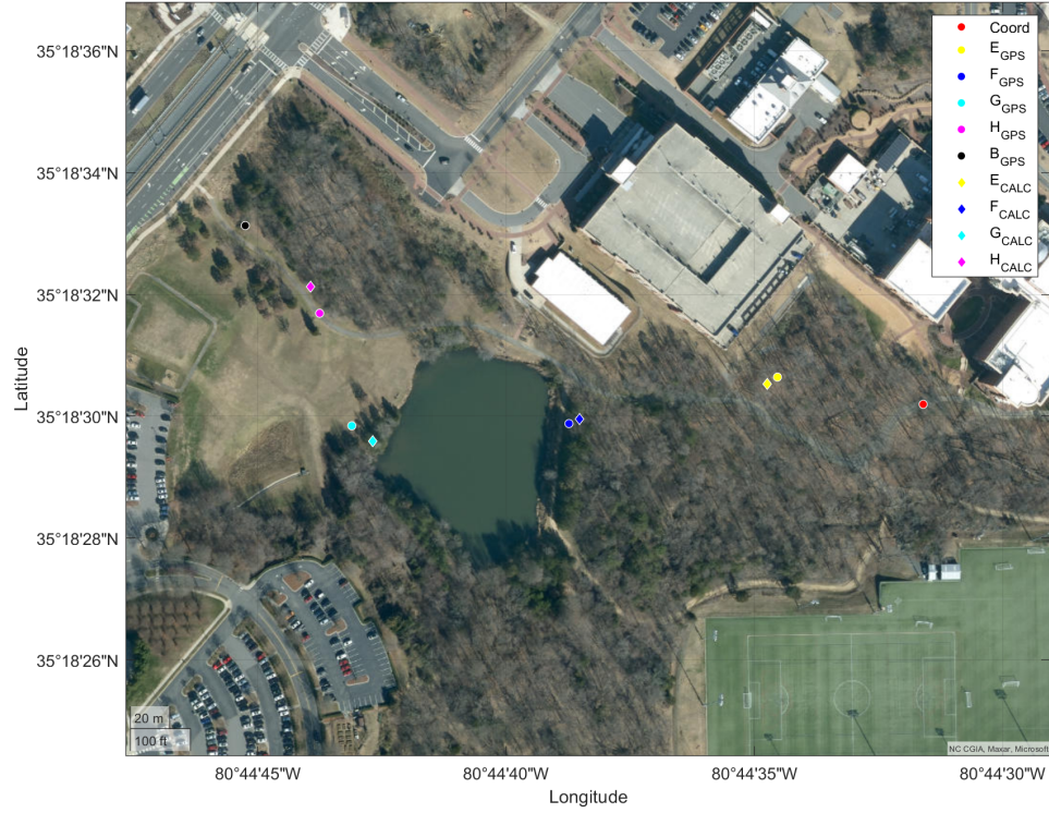
Figure 4.35: Outdoor trial 1 BreadCrumb initial location results. Mean Error: 10.1031 meters.
