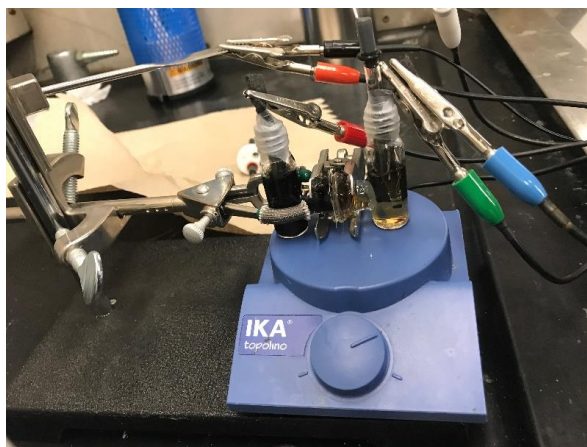
FIGURE 1.22. Symmetrical H-cell set up with the CF WE (blue/green connection), Ag/AgCl RE (white connection), and CF CrE (red connection) connected to a Gamry 1000E potentiostat, separated by a Selemion AMV anion exchange membrane, and sealed with a DuPont Kalrez perfluoroester O-ring.
