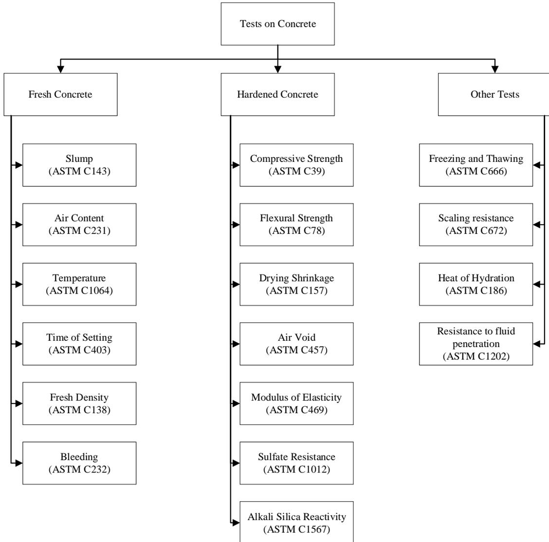
FIGURE 2.7 Standard tests for evaluating the suitability of ASCM on concrete (ASTM C1709-18)
