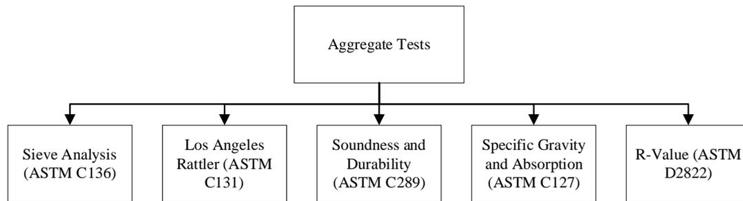
FIGURE 2. 6 Standard Test for evaluating the suitability of aggregate in concrete.
