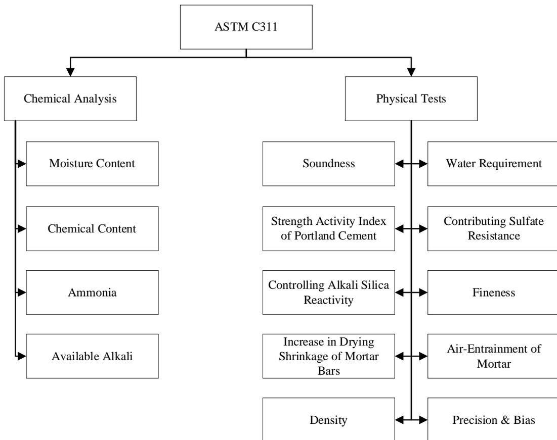
FIGURE 2.8 Standard Tests for Testing Fly Ash or Natural Pozzolans for Use in PCC.
