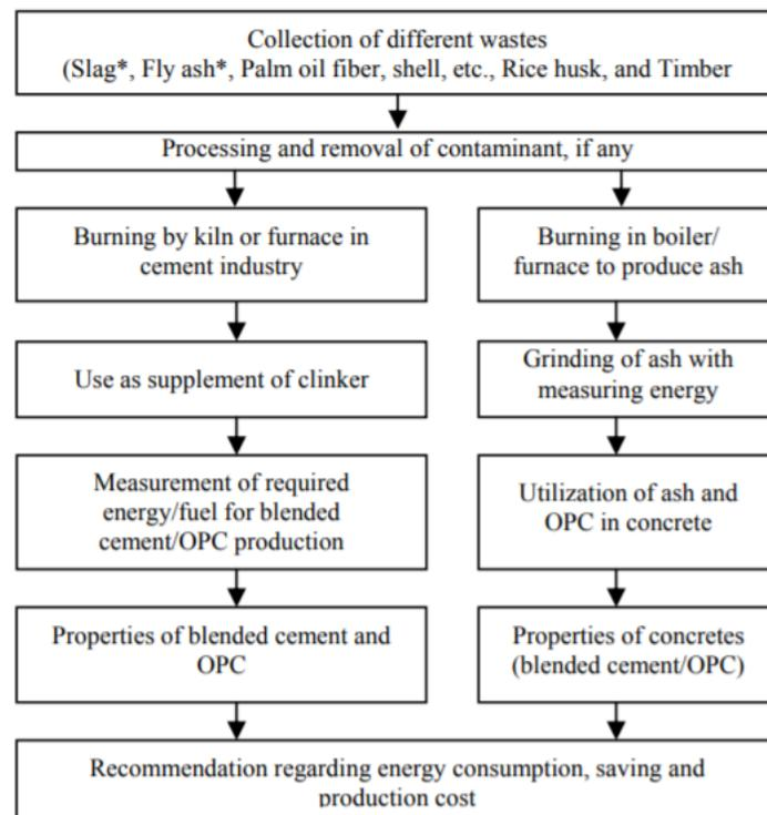
FIGURE 1.1 Utilization of wastes in cement and concrete as an energy saving approach (Karim et al. 2011).
