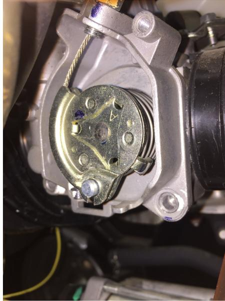
Figure 3.8: Throttle wire and spring at the air valve side.
