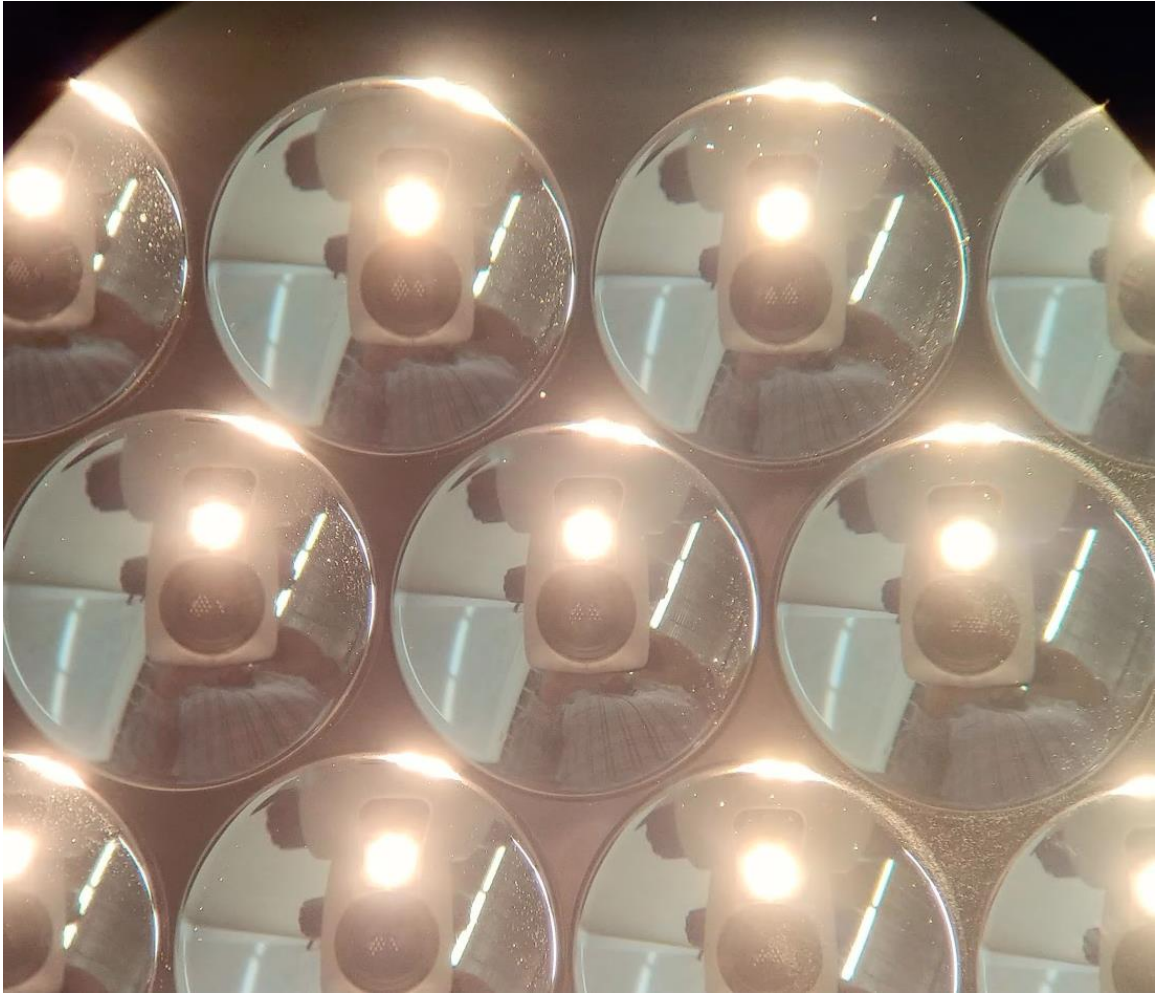
FIGURE 32: FLIR Hex Packed Array 2nd Finish Cut, Outer Lenses Above Center
