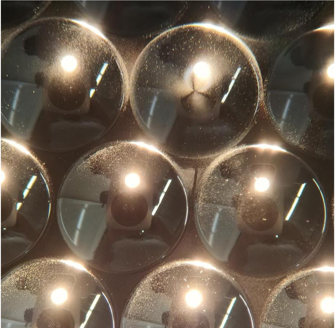
FIGURE 29: FLIR Hex Packed Array 1st Finish Cut, Central Lenses
