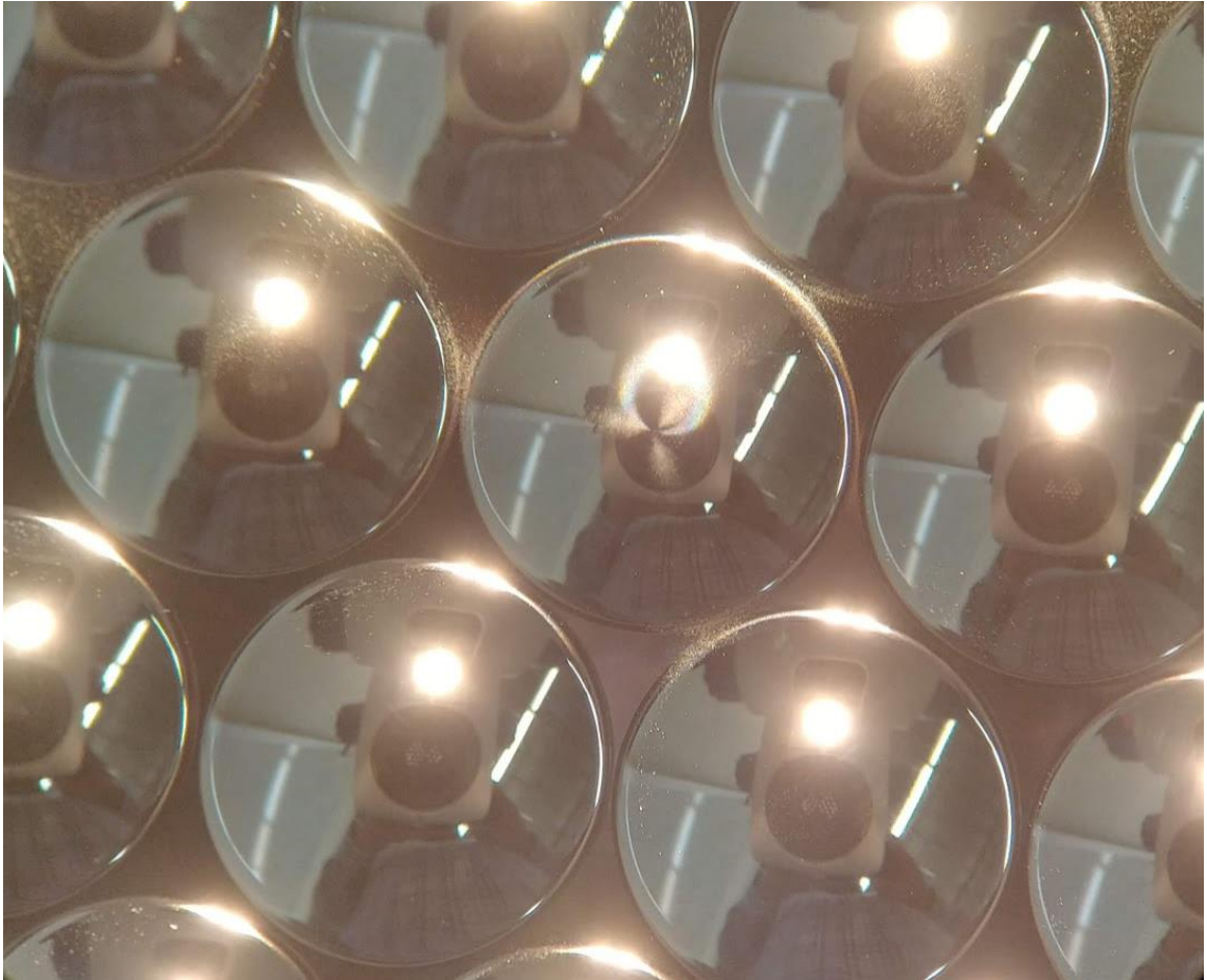
FIGURE 31: FLIR Hex Packed Array 2nd Finish Cut, Central Lenses
