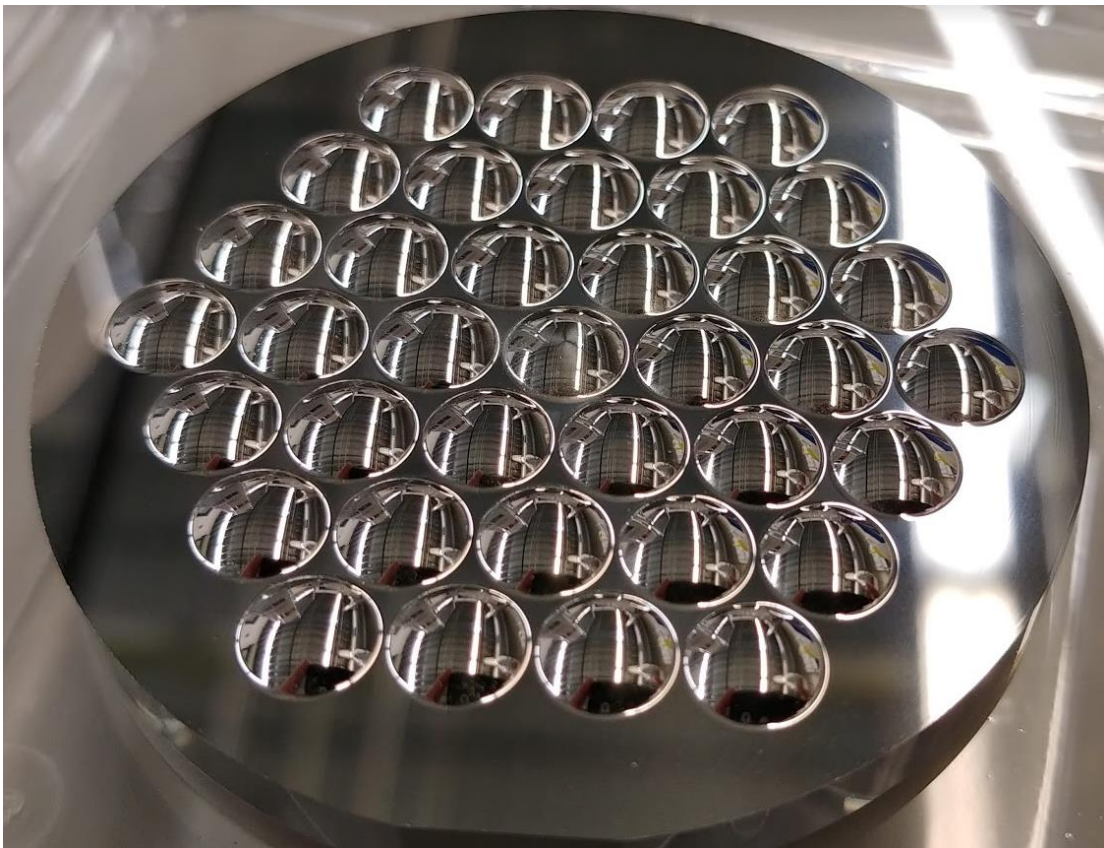
FIGURE 28: FLIR Hex Packed Array 1st Finish Cut
