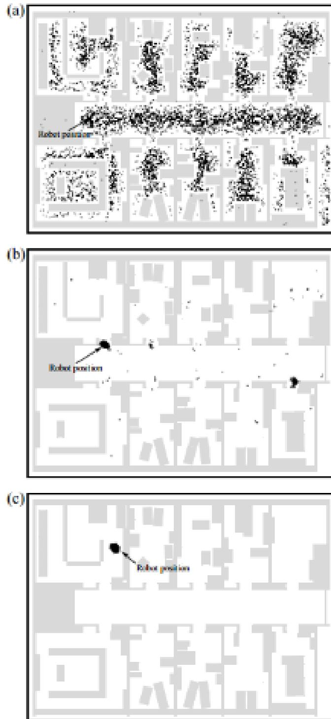
Figure 3.5: Localization using particle filter. Figure (a) demonstrates particles being propagated everywhere uniformly. Figure (b) shows 3 clusters converged due to the symmetrical nature of the passage. Figure (c) shows particles being converged at one point after the robot encountered structurally unique features [20].
