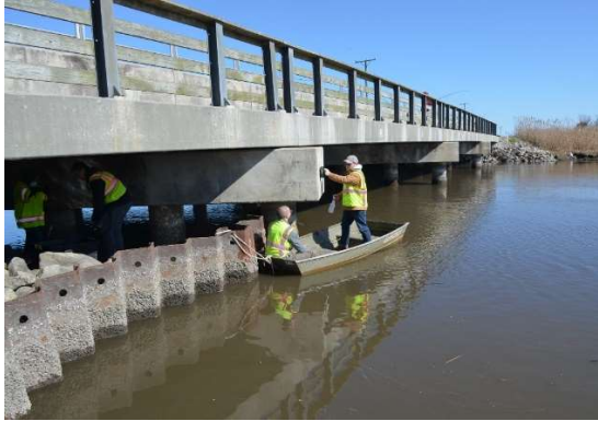
Figure A1.35. Center: Using iCOR On Side Face of Interior Bent; Left of Center: Drilling for Powder Samples on Interior Face of Interior Bent.
