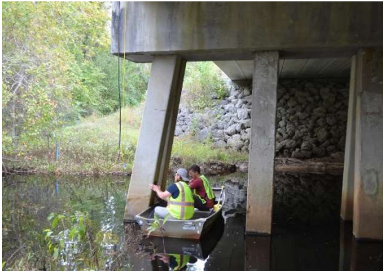
Figure A1.16. Research Team Utilizing Boat to Perform iCOR Testing of Piers.
