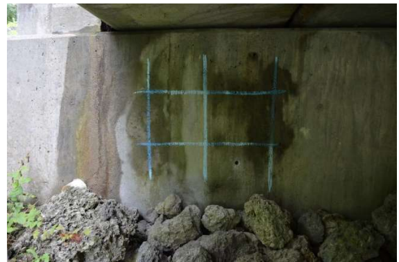
Figure A1.13. Location Of iCOR Test Grid and Powder Sample Collection; East Side of End Bent.
