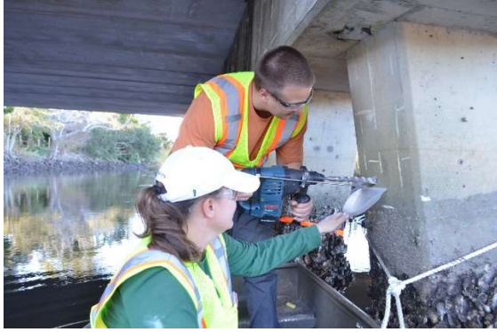
Figure A1.26. Research Team Using Drill to Collect Powder Samples from Pier.
