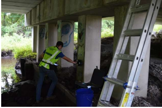
Figure A1.4. Measuring Corrosion Rate and Surface Resistivity (iCOR) At Center Pier.
