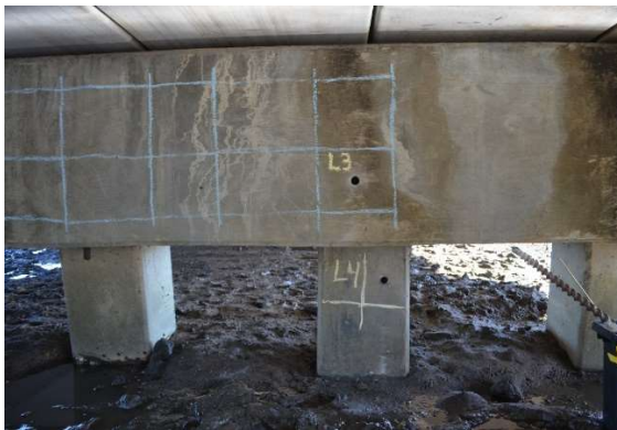
Figure A1.28. Testing Grid For iCOR And Powder Sample Locations 3 And 4.
