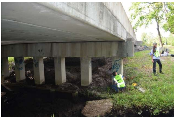
Figure A1.2. Research Team Using Pachometer To Locate Rebar.
