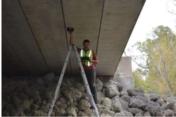
Figure A1.20. Research Team Using iCOR To Test Underside of Cored Slabs.
