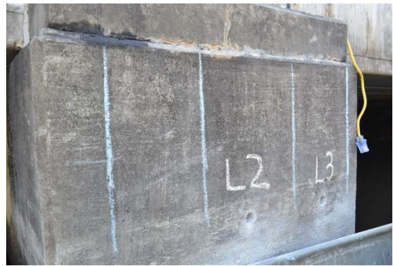
Figure A1.34. Location of Powder Samples And iCOR Grid on Side Face of Interior Cap.
