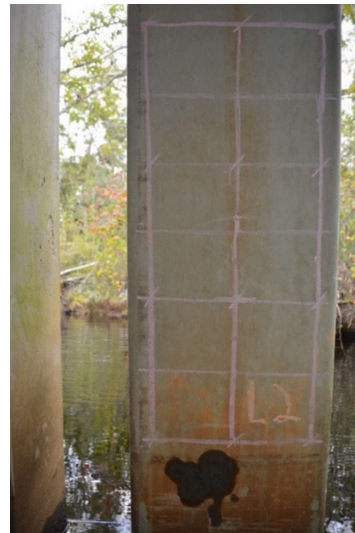
Figure A1.19. Location 2 Of iCOR Testing Grid and Powder Sampling Location.
