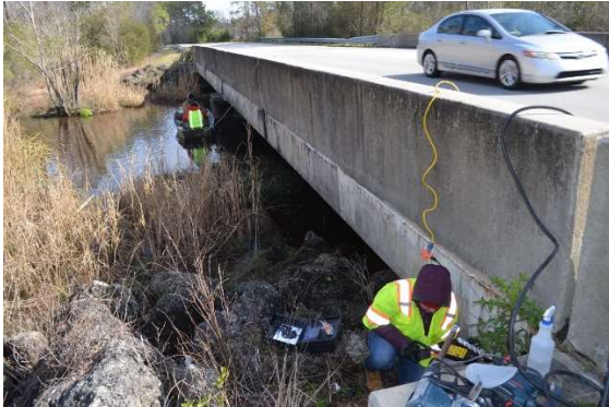
Figure A1.31. Lower Right: Using Pachometer To Locate Steel in Wing Wall; Left of Center: Performing iCOR Testing on Face of Cap from Boat.
