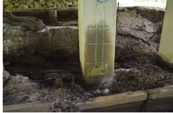
Figure A1.5. Location of iCOR Test Grid and Powder Sample Collection at Center Pier.
