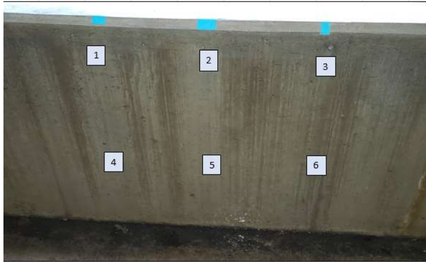
Figure 3.1. Test Grid for iCOR versus Resipod Comparison Study.
