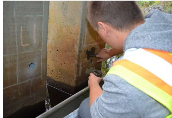
Figure A1.17. Research Team Filling Powder Sample Holes After Collection.
