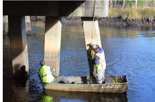
Figure A1.22. Research Team Using Pachometer To Identify Steel Location in Piers.
