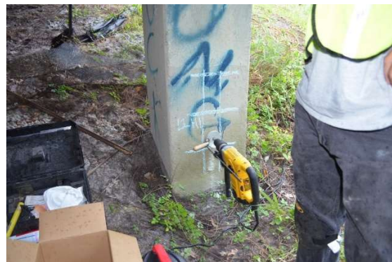
Figure A1.3. Collection of Powder Samples from West-Most Pier.
