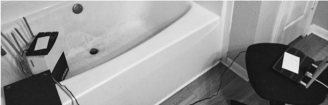
Figure 13 Experimental setting for CSI data collection using two routers.
