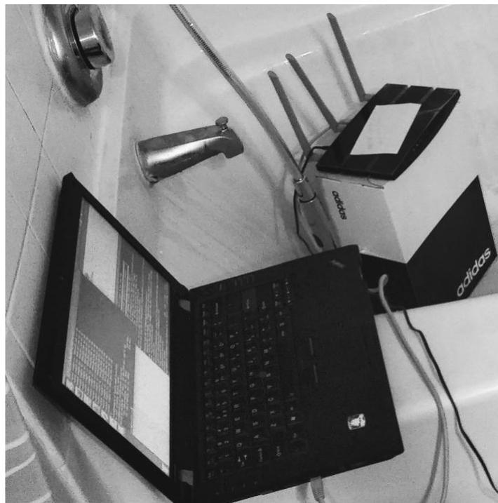
Figure 14 CSI data collection setting, showing the shower head, router and the laptop used.
