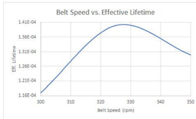
Figure 4.6: Belt Speed vs Minority Carrier Lifetime [18]
