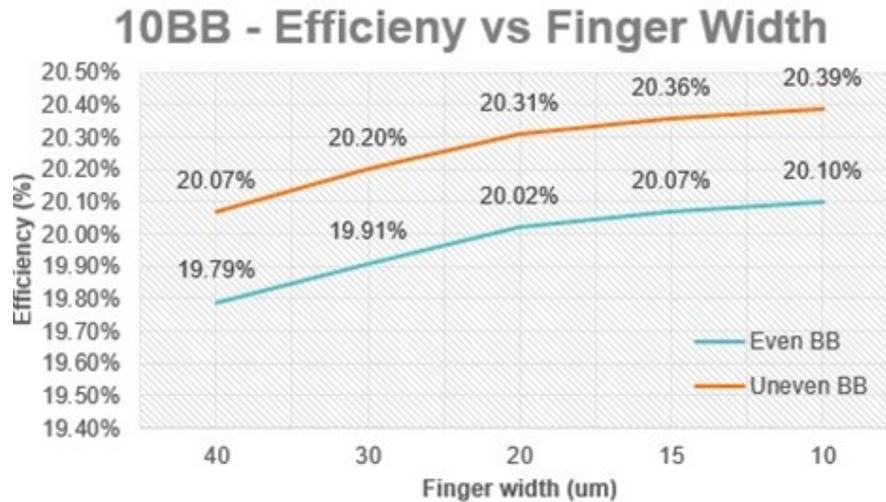
Figure 3.9: 10BB - Efficiency as a function of NTPF width with EBB and UEBB
