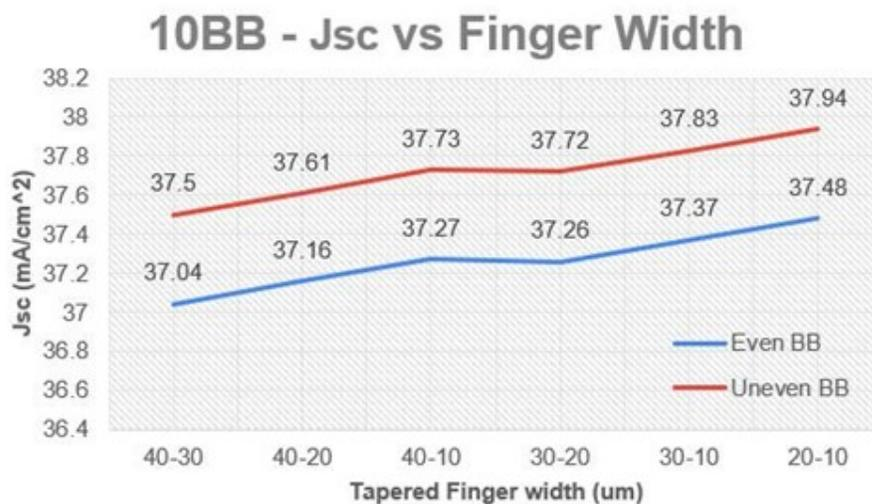
Figure 3.14: 10BB - Short Circuit Current as a function of TPF width with EBB and UEBB
