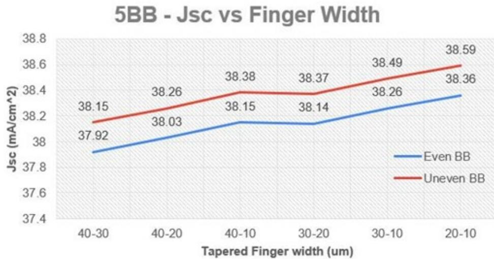
Figure 3.7: 5BB - Short Circuit Current as a function of TPF width with EBB and UEBB
