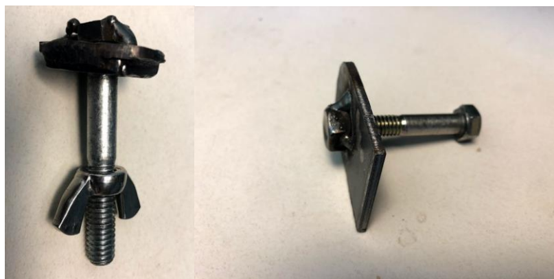
FIGURE 3. 3 Screw Arrangements for fixing 2"x4" bar
