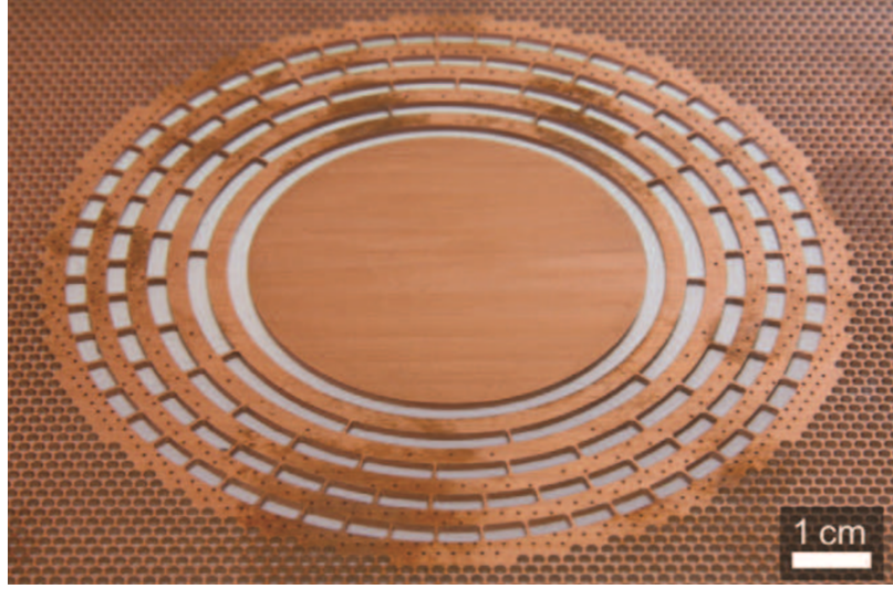
Figure 1.2: Example of fabricated thermodynamic heat cloak [2]
