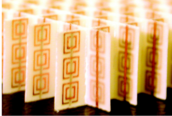
Figure 1.6: Square split ring resonators periodically arranged to perform as a left-handed material [7]
