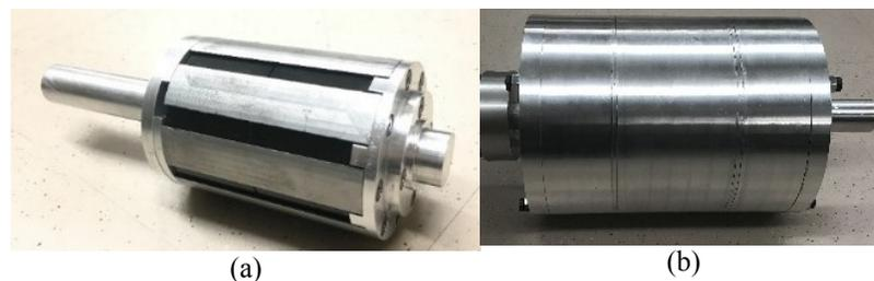
Figure 3-9. (a) High-speed inner rotor assembly (b) fully assembled MG
