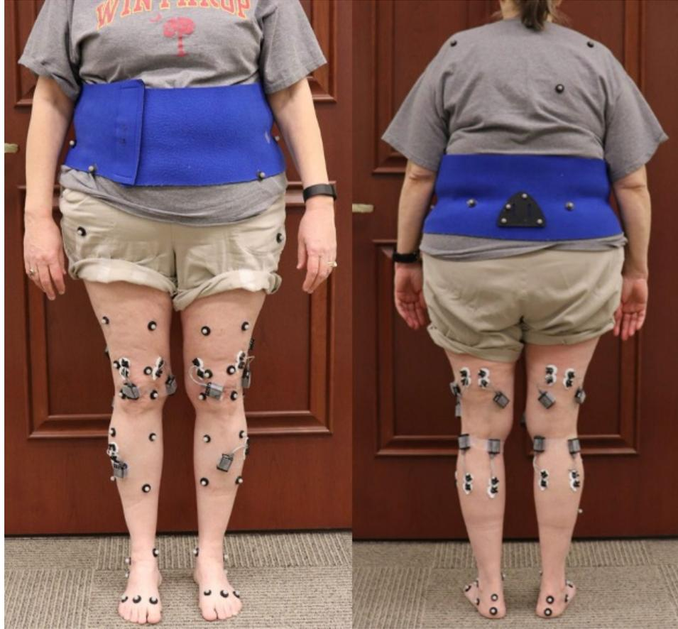
FIGURE 3 Anterior and posterior views of TKA subject with motion capture markers attached to the body.
