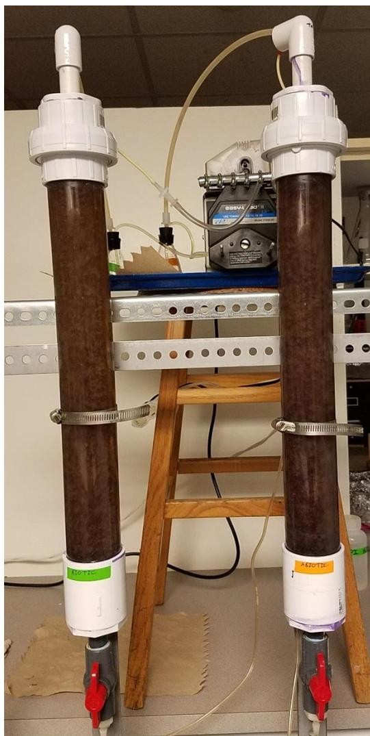
Figure 3. Plug flow column reactors (Left, biotic and right, abiotic)
