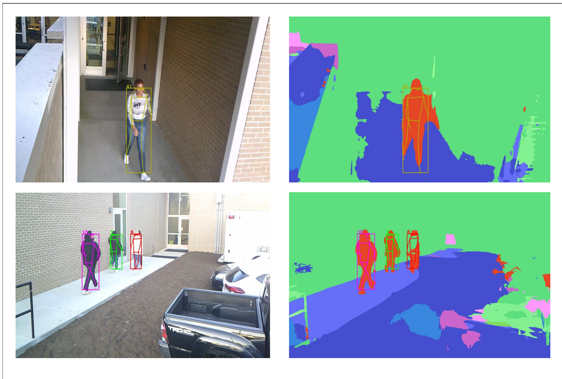
Figure 4.2: EfficientHRNet Pose Estimation and Segmentation in Vision pipeline. Left: Pose Estimation, Right: Segmentation.
