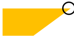
Figure 4.7: Side view of diamond. Cutting edge sharpness refers to the nanometer-scale radius of the cutting edge emphasized by the black circle.
