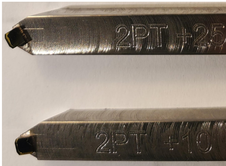
Figure 7.2: Custom tools with the diamond blank brazes on at an angle.
