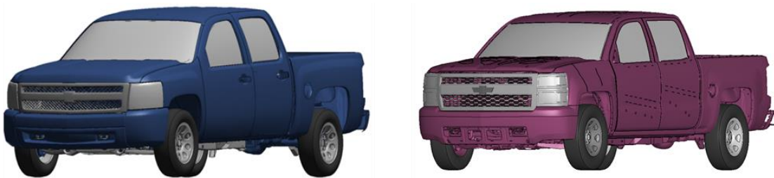
Figure 3.3: The FE models of a 2007 (left) and a 2014 (right) Chevy Silverado quad-cab pick-up truck.
