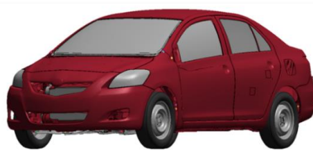
Figure 3.2: The FE model of a 2010 Toyota Yaris passenger sedan.
