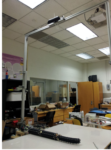
Figure 53: Experimental set up with a table top OctArm, overseen by an overhead Microsoft Kinect.
