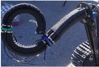
(e) OctArm developed by Jones and Walker [99]
