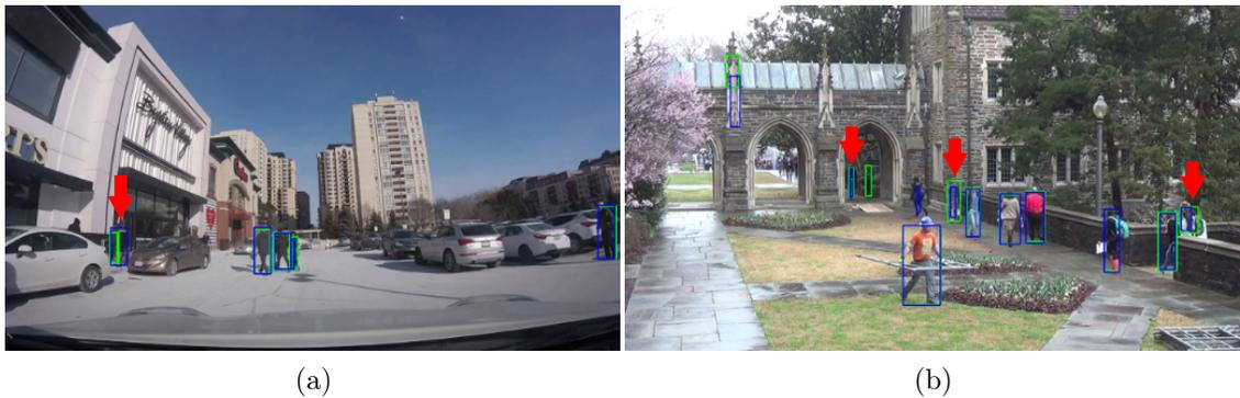
Figure 3.8: The impact of accuracy reduction on video frame modification by the latency controller for JAAD (a) and DukeMTMC (b). Green and blue bounding boxes indicate pedestrian detections on unmodified and modified video frames respectively. The video frames experience an accuracy loss of  $\approx 3\%$  for JAAD and  $\approx 4\%$  for DukeMTMC respectively. The red arrows show the resulting detection errors.
