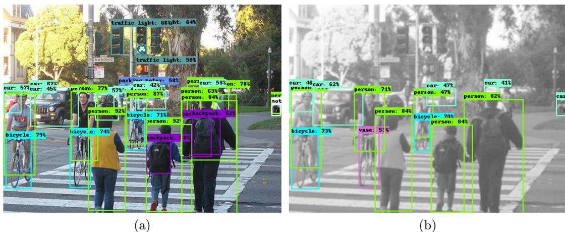
Figure 6.5: Visual impact on object detections before and after the application of tuning knobs. (a) unmodified video frame and (b) video frame after applying knobs - colorspace modification, denoising, contrast stretching and gaussian filtering.
