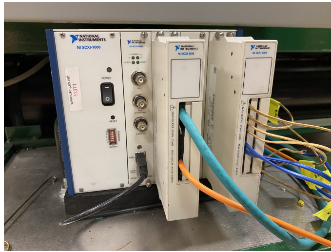
Figure 1.15: The SCXI sitting below the control box on the UNC Charlotte hypersonic wind tunnel
