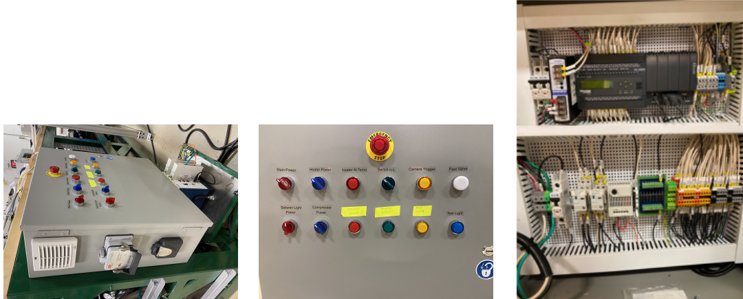
Figure 1.14: This figure displays the control box secured to the frame of the UNC Charlotte wind tunnel
