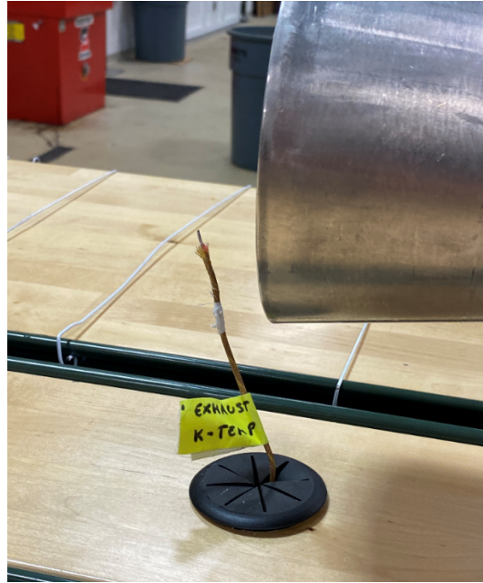
Figure 1.13: This figure is an image of the thermocouple that emerges from under the surface of the hypersonic wind tunnel close to and downstream of the diffuser of the wind tunnel.
