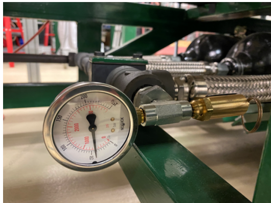
Figure 1.11: This is an image of the pressure gauge tapped into the Manifold
