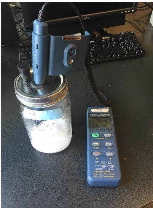
Figure 3. Relative humidity jar and measurement device
