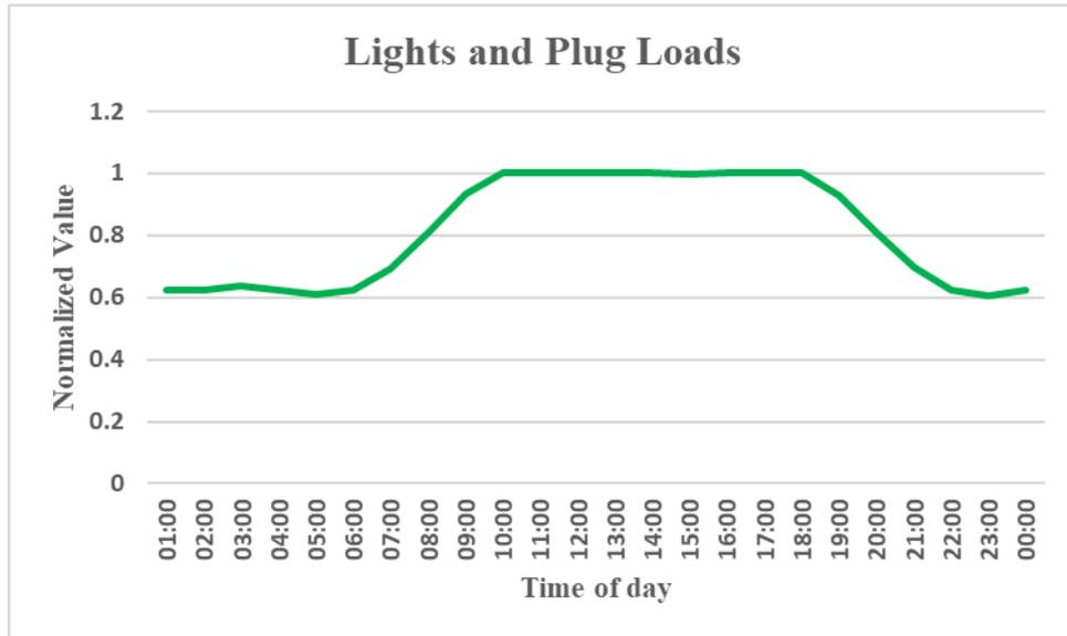
FIGURE 2.3: Demand profile for lights and plug loads
