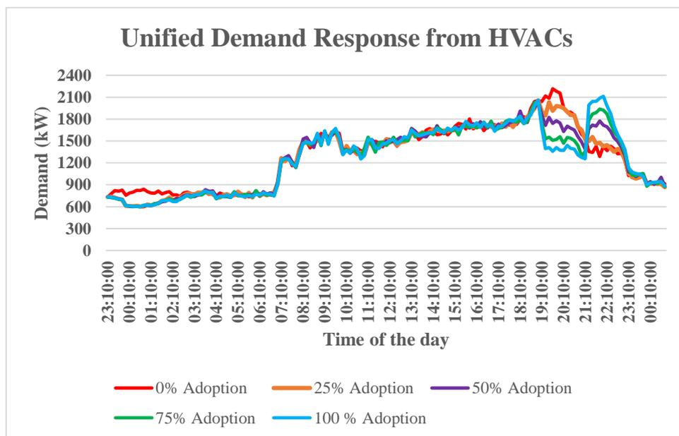
FIGURE 3.9: Unified signal for DR from HVACs
