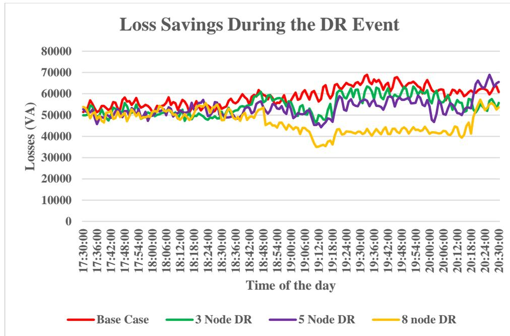
FIGURE 4.10: Impact of DR on system losses
