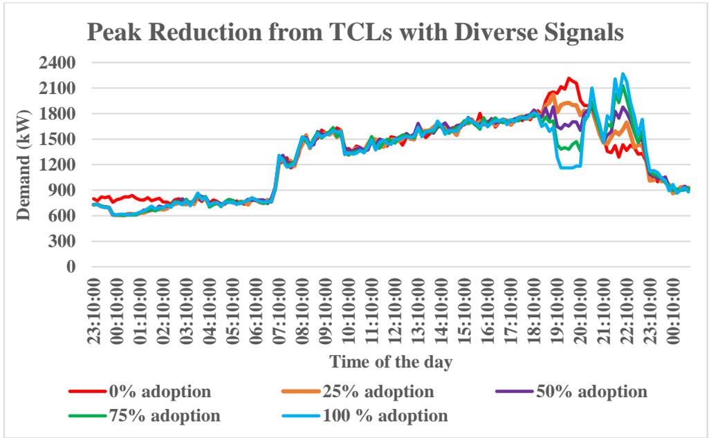
FIGURE 3.6: Rebound mitigation using diverse signals
