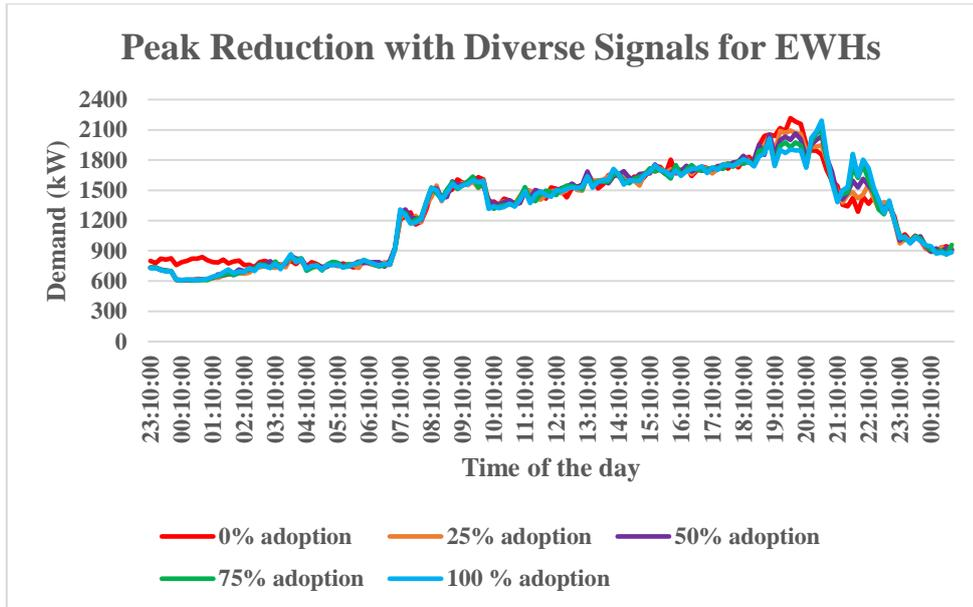
FIGURE 3.18: Peak reduction with diverse signals for EWHs
