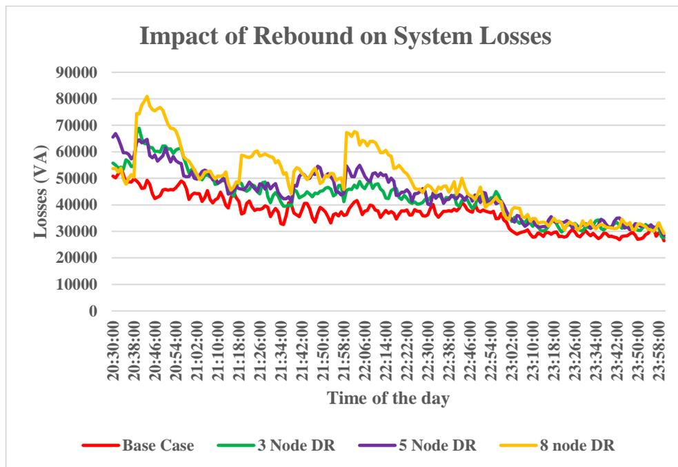
FIGURE 4.11: Impact of rebound on system losses
