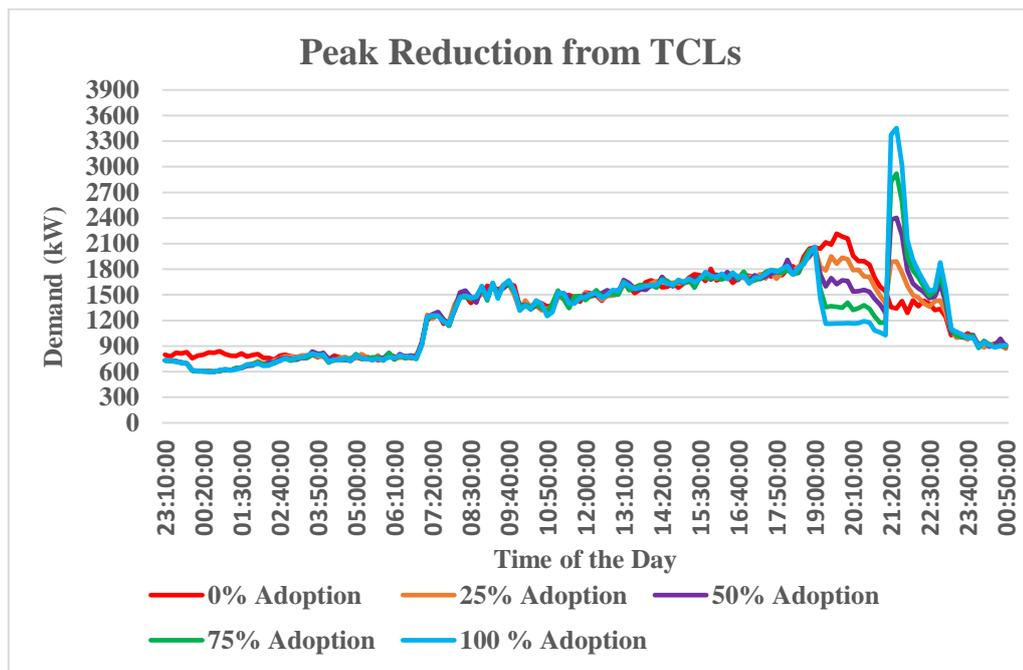
FIGURE 3.4: Peak reduction using TCLs
