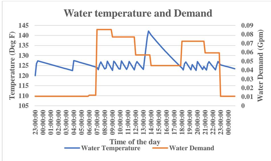
FIGURE 3.26: Water temperature and demand from water heater
