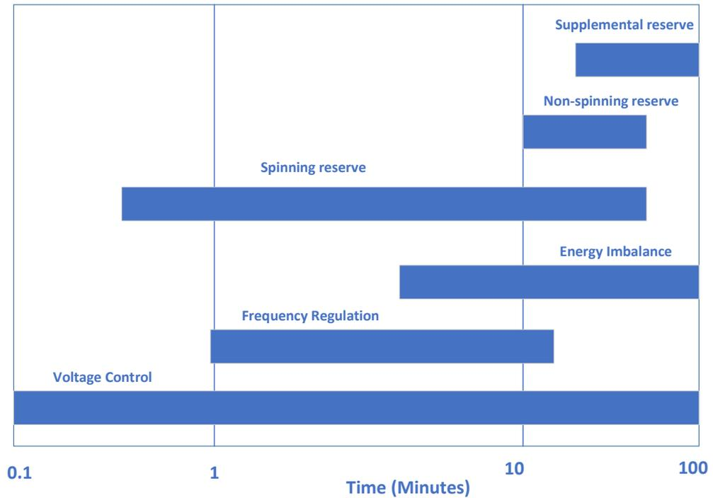
FIGURE 4.1: Ancillary Services based on response speed and duration
