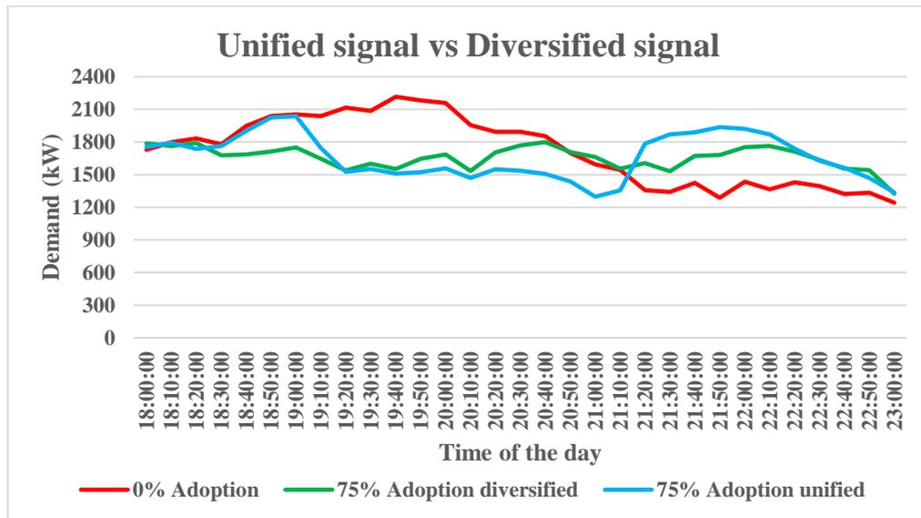
FIGURE 3.13: Unified vs Diversified signal for HVACs
