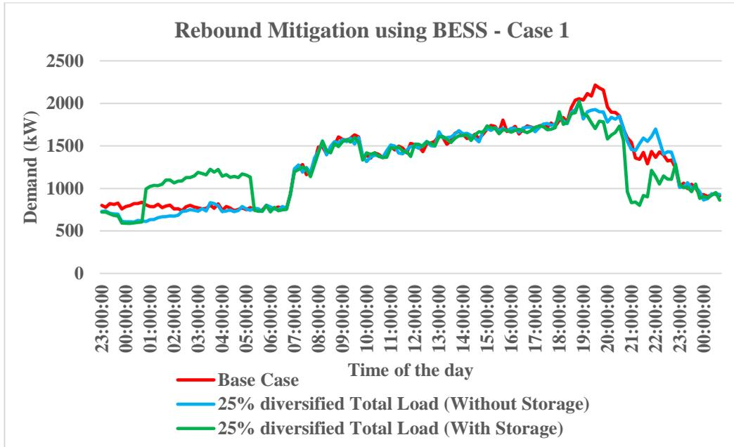
FIGURE 3.22: Rebound mitigation and load leveling for 25% DR and 25% BESS adoption scenario
