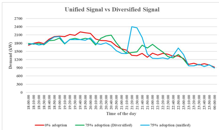
FIGURE 3.20: Unified vs diversified signals for EWHs
