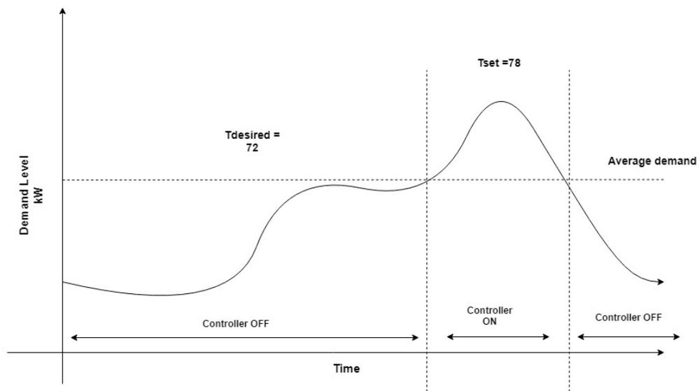
FIGURE 3.1: Graphical representation of cooling mode controller operation
