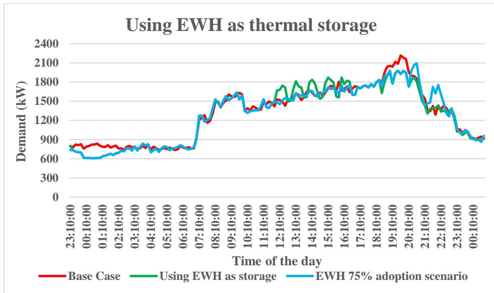
FIGURE 3.25: Using EWH as thermal energy storage
