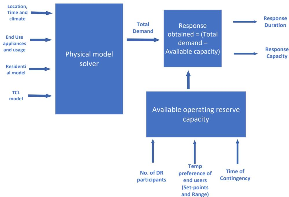
FIGURE 4.3: Operating reserves capacity architecture
