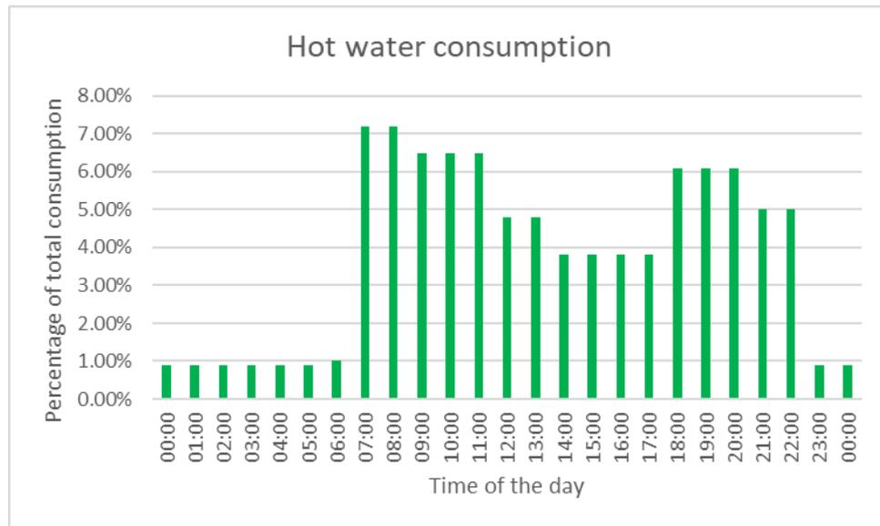
FIGURE 2.4: Hot water consumption for one day [7]
