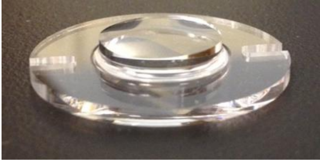
Fig. 3.1: One of the two freeform elements for the first variable beam shaper, fabricated using diamond milled approach on the Moore Nanotech ® 350 FG.
