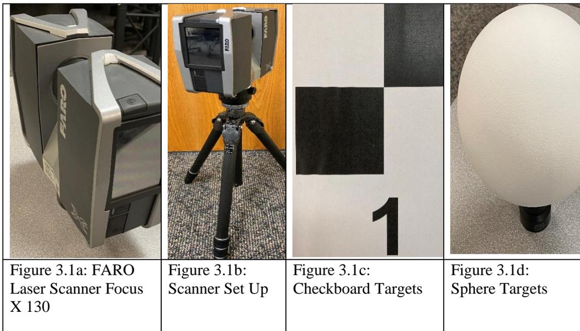
FIGURE 3.1: Scanner and Targets
