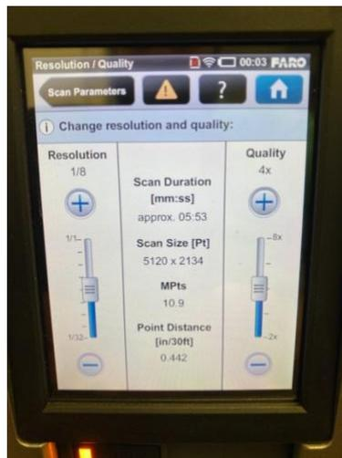
FIGURE 3.2: Scanner Resolution and Quality Set Up
